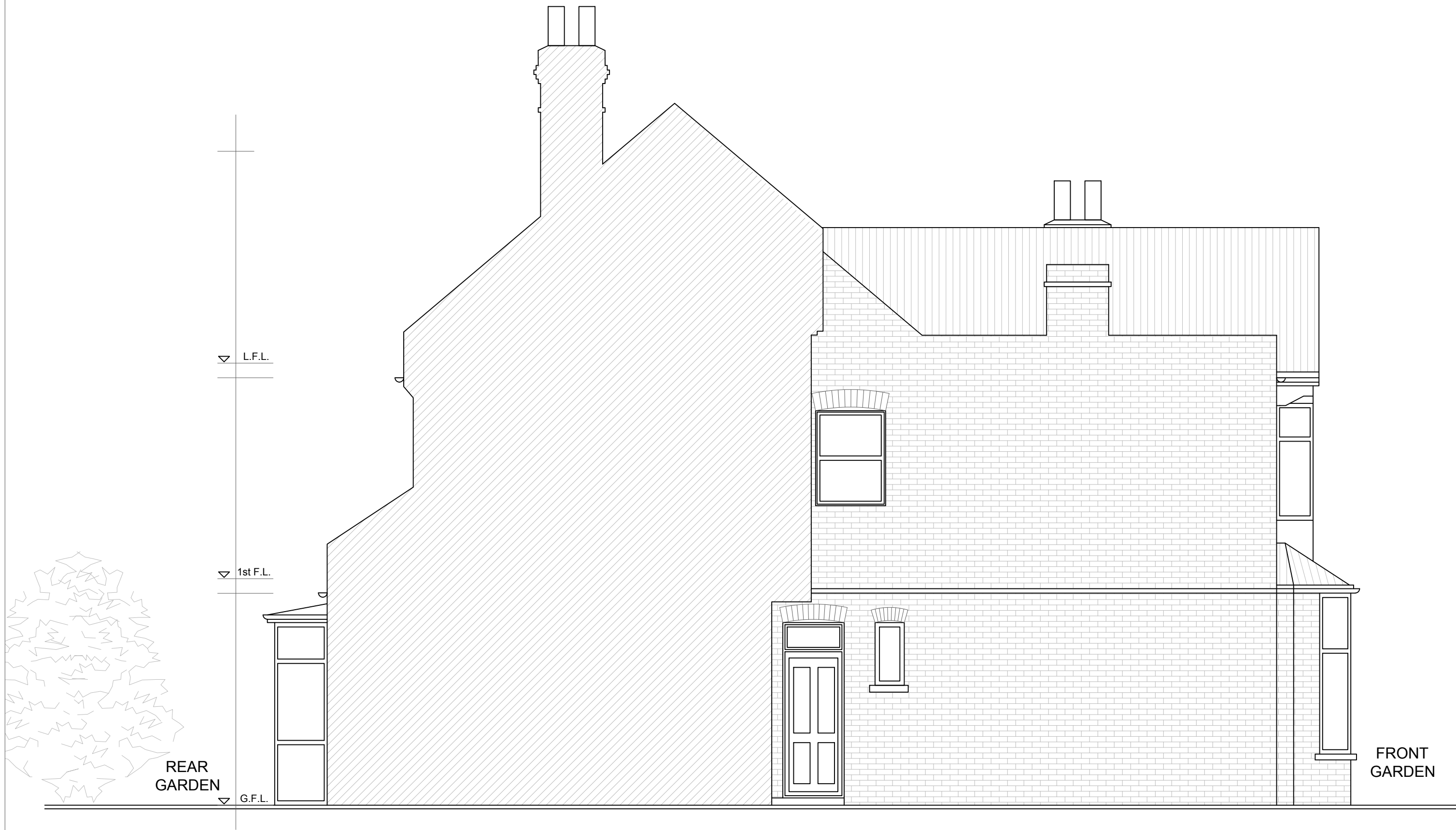
EXISTING LEFT HAND SIDE ELEVATION
