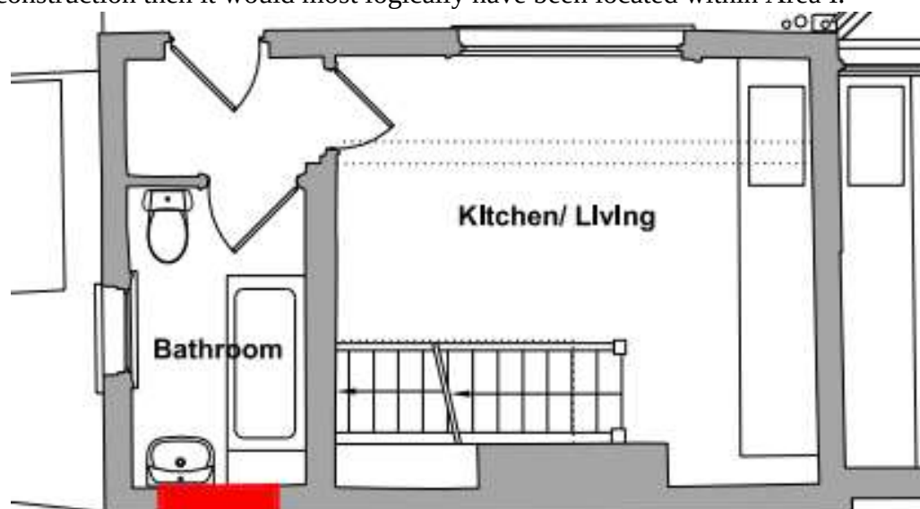
Figure 154: Ground floor plan of 9a Muswell Hill, with blocked window marked in red.
