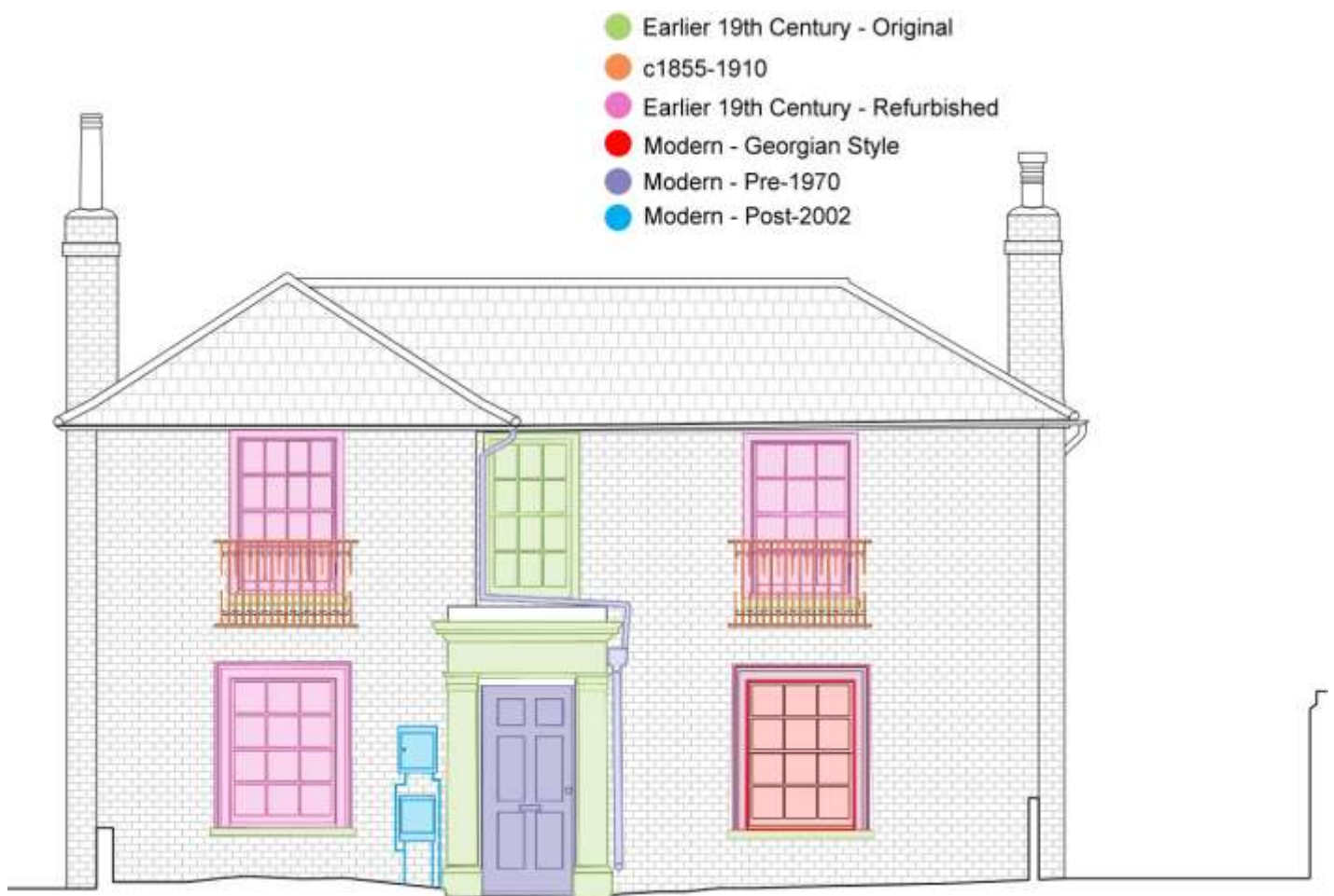
Figure 193: Front Elevation edited to indicate dating phases for features.
