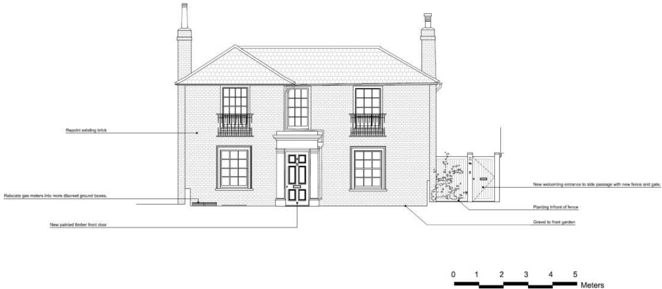
Figure 198: Proposed Front (East) Elevation, with works annotated. Produced by Studio Elephant Architects. Drawing No. 2200-PE-F. Rev. P1 (06/02/26)
