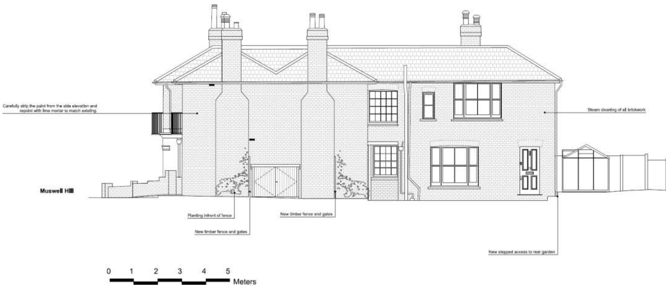
Figure 199: Proposed Side (North) Elevation, with works annotated. Produced by Studio Elephant Architects. Drawing No. 2201-PE-S1. Rev. P1 (06/02/26)
