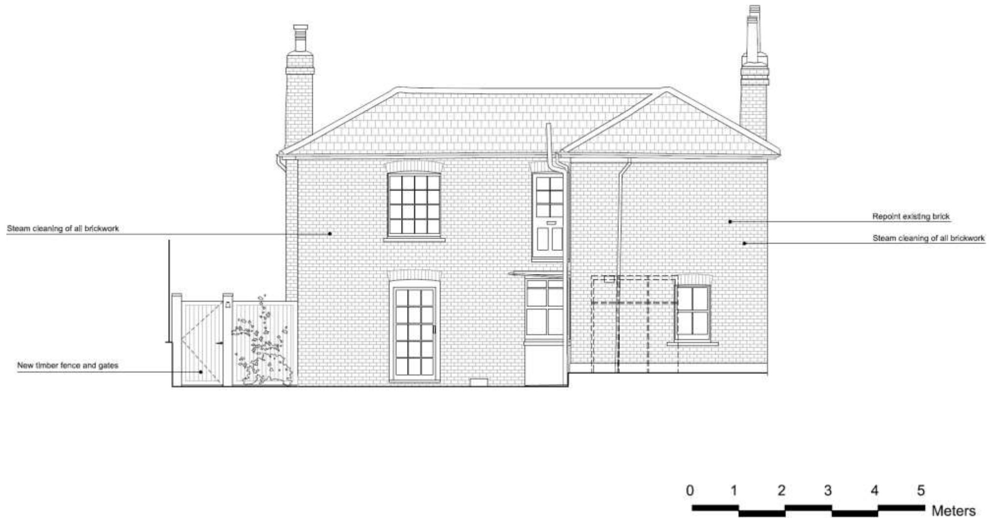
Figure 200: Proposed Rear (West) Elevation, with works annotated. Produced by Studio Elephant Architects. Drawing No. 2202-PE-R. Rev. P1
