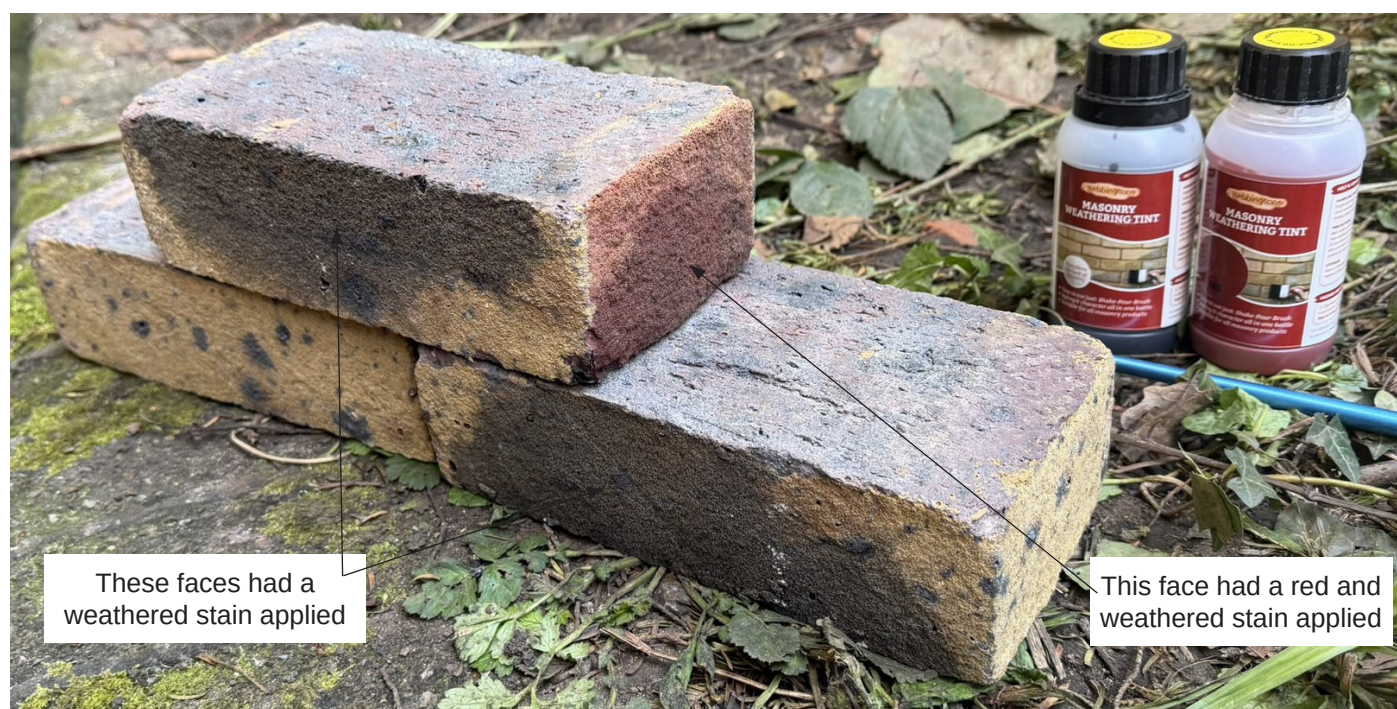
Photograph G – Use of brick tinting to create a better match
