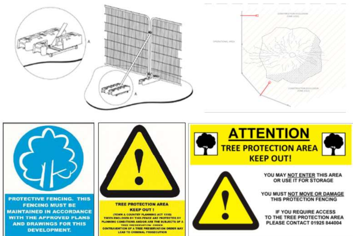
Image 3.17b – example of tree protection measures
