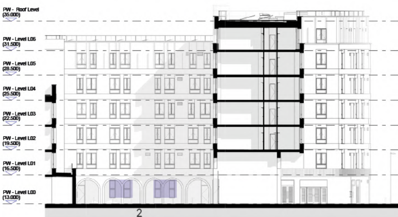
FIGURE 35. Consented Scheme- Section through Western Courtyard
