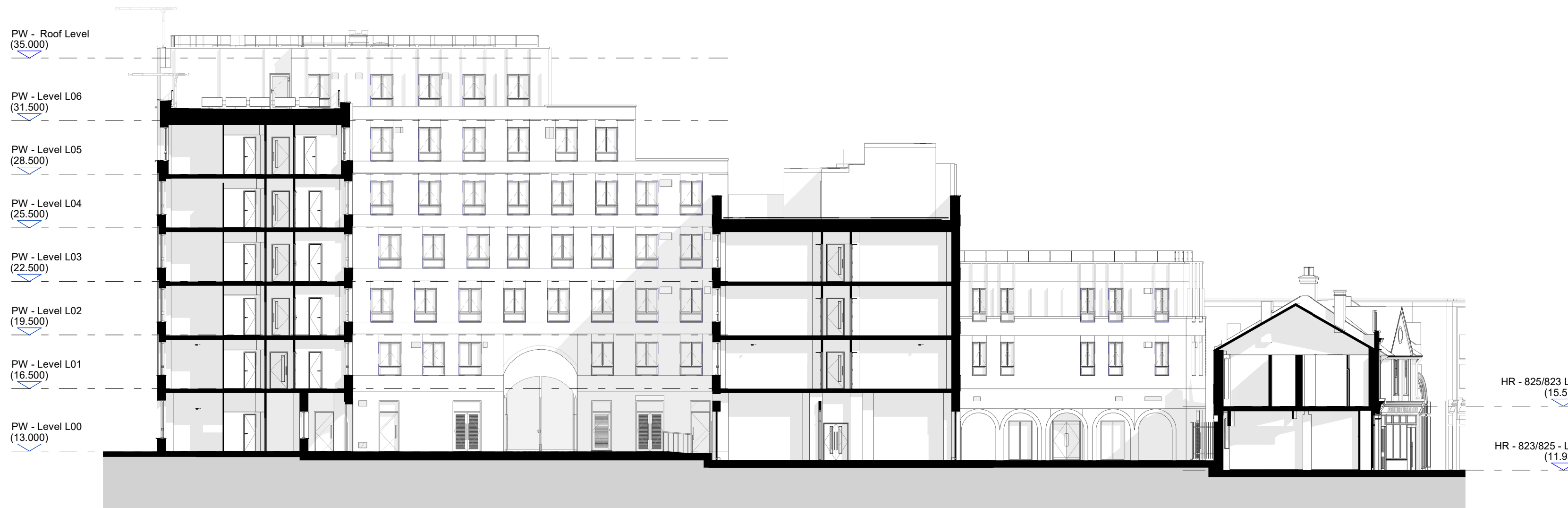
E 82611 SECTION 2 - WEST EAST THROUGH COURTYARD SCALE 1 : 200
