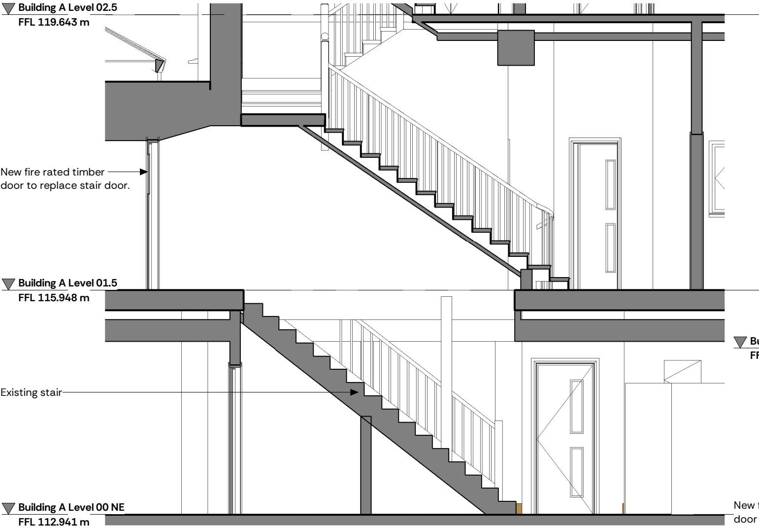
Section Thro' Existing Stair Scale 1 : 50
