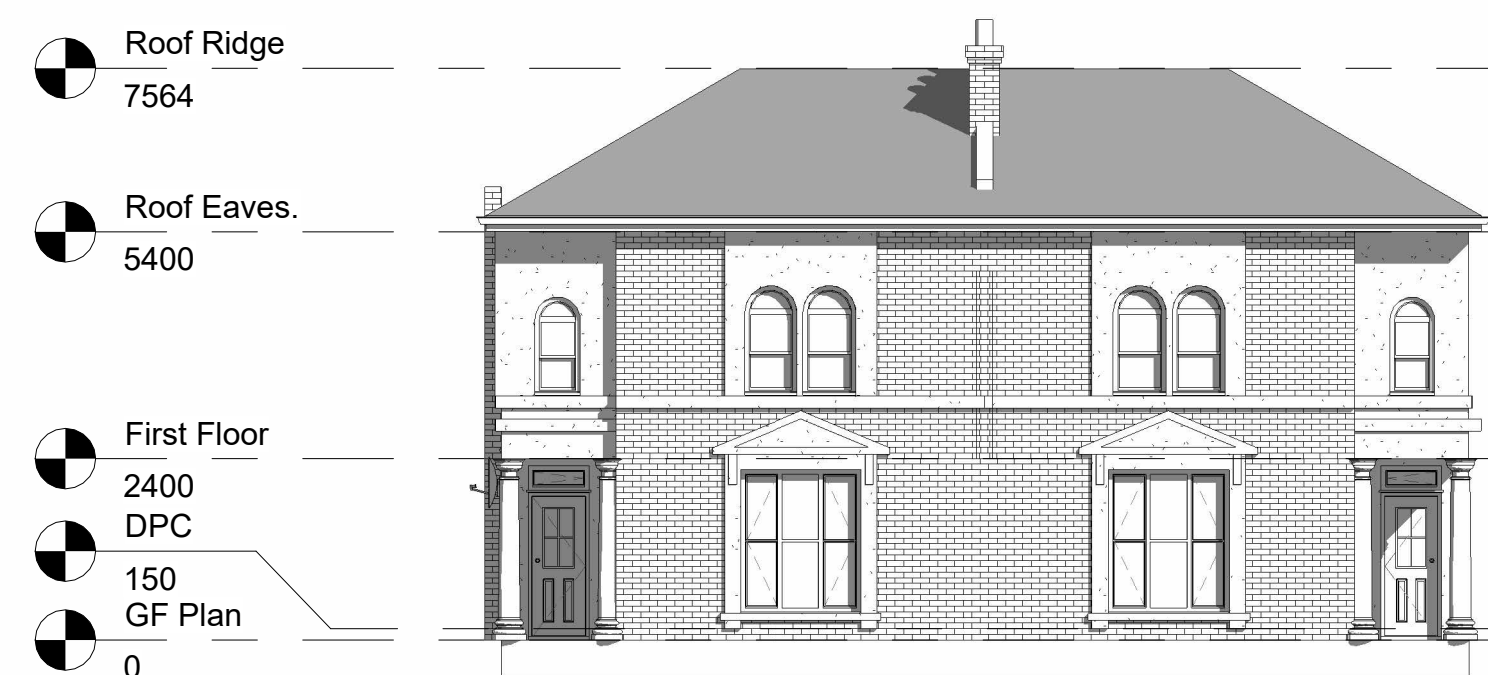
4 South Elevation Existing 1 : 100
