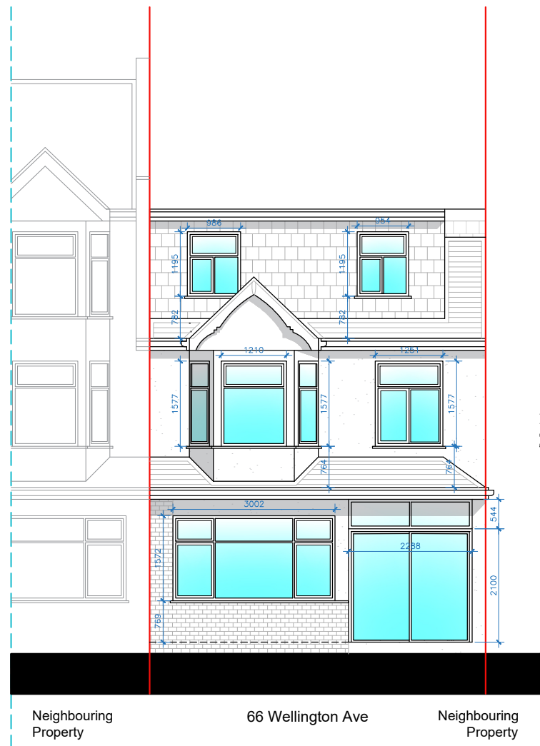
NORTH-EAST ELEVATION (FRONT VIEW)
