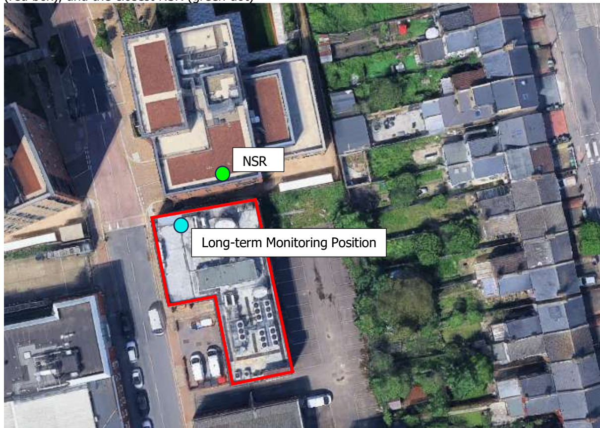
Figure 4: Google image showing the long-term noise monitoring location (blue dot), the site location (red box), and the closest NSR (green dot)
