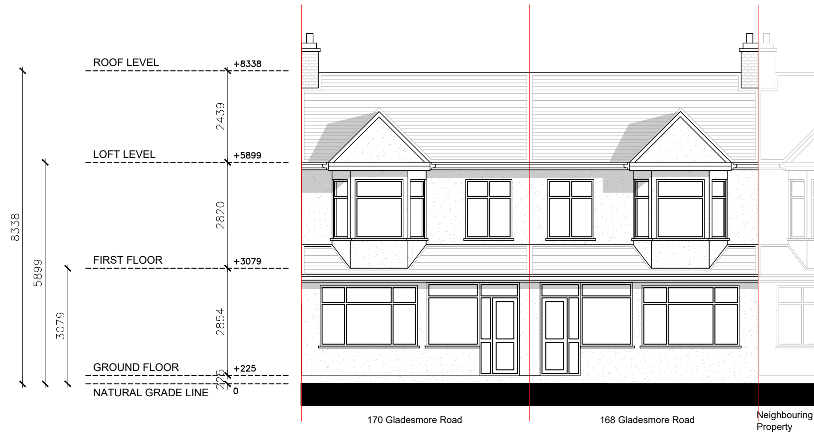
NORTH-EAST ELEVATION (FRONT VIEW)
