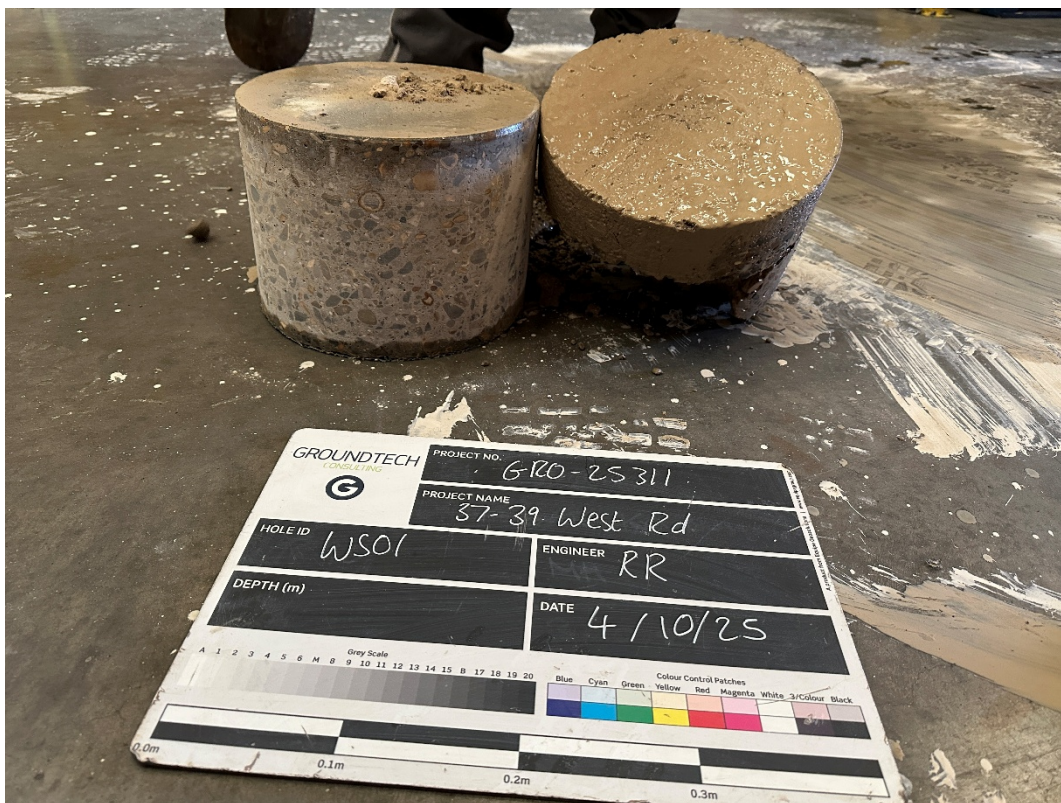
Photograph 8 – Double concrete slab encountered in WS01 to 0.43m begl.
