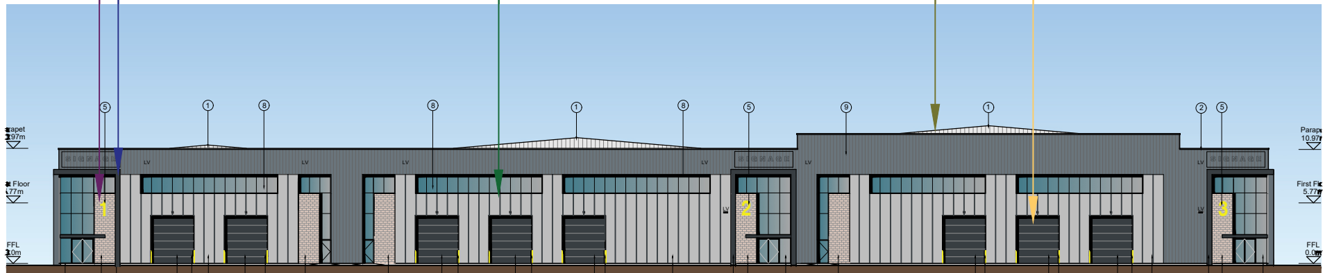
Metal, trapezoidal profile roof cladding - Goosewing Grey (RAL 7038) with coordinated polycarbonate rooflights or equal in specification, appearance and colour.
