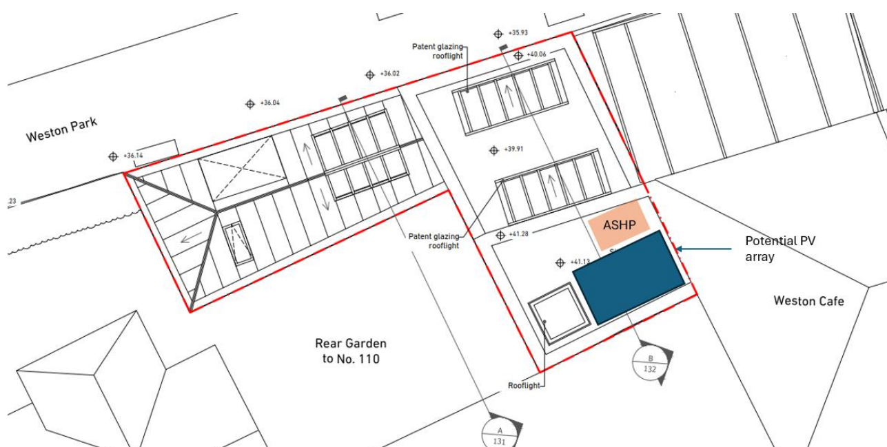
Figure 3: Roof plan mark-up of potential ASHP external unit positioning and solar PV array.
