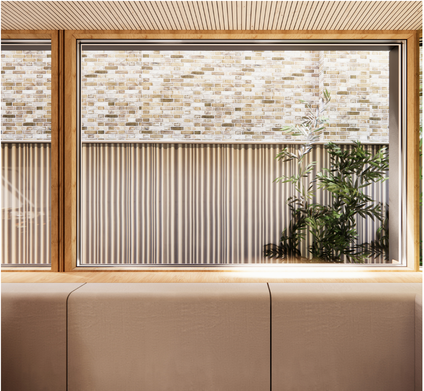
Figure C - 3D visualisation showing proposed boundary wall as viewed from principal living space, with Friesland formliner finish to lower retaining wall, bullnose coping stone, and rebuilt reclaimed brick wall above.
