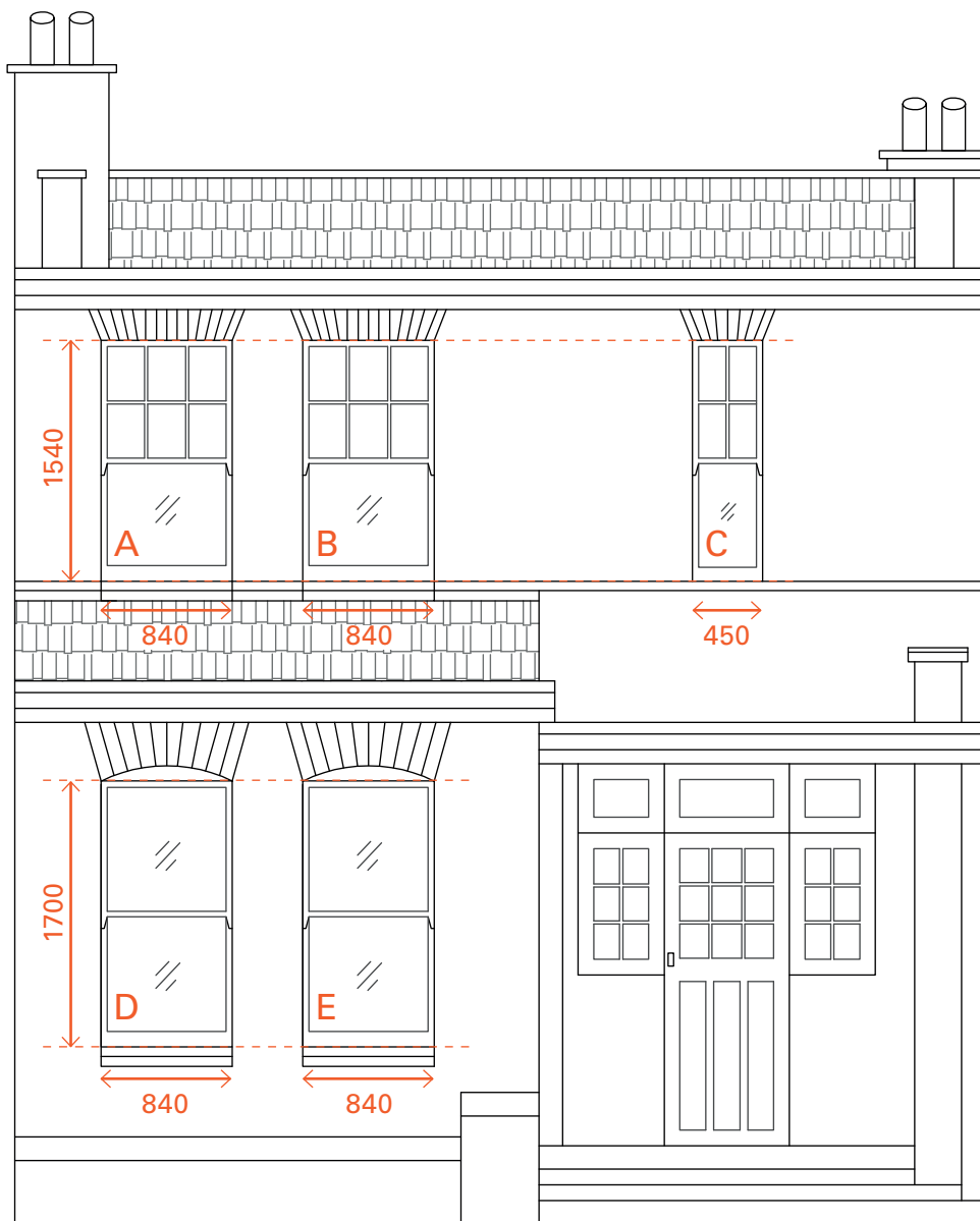
EXISTING FRONT ELEVATION
