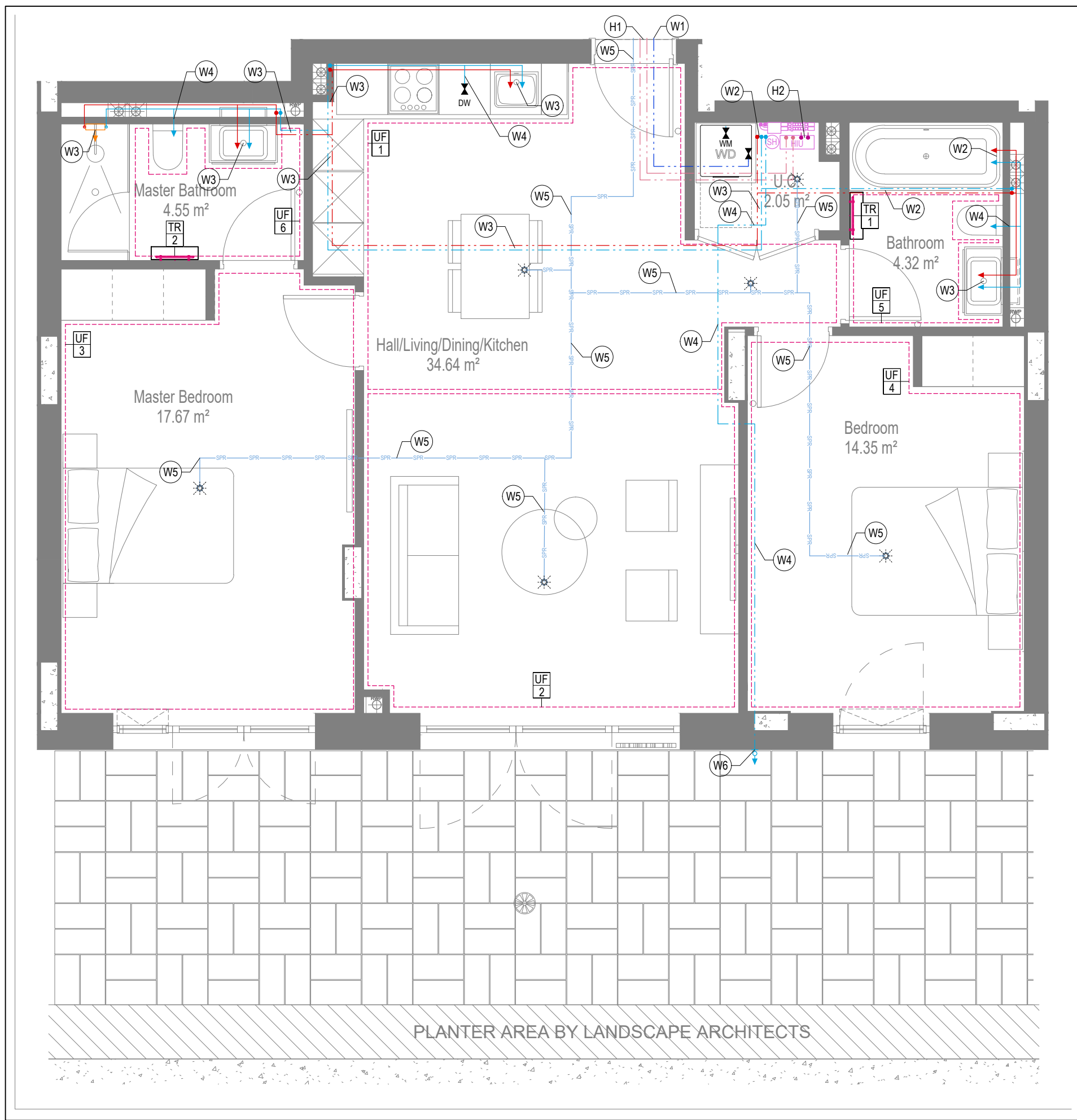
WATER AND HEATING LAYOUT
