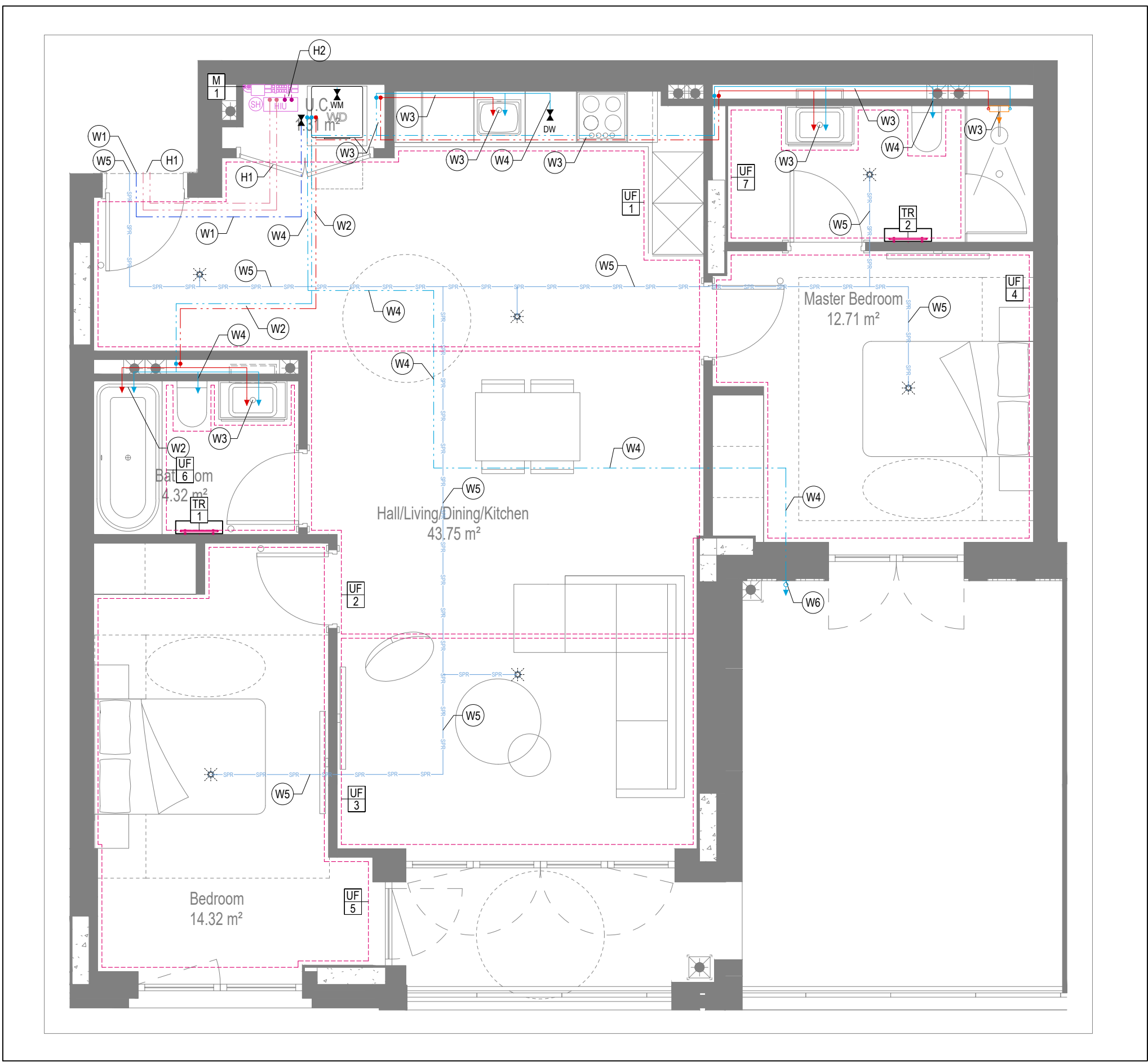
WATER AND HEATING LAYOUT
