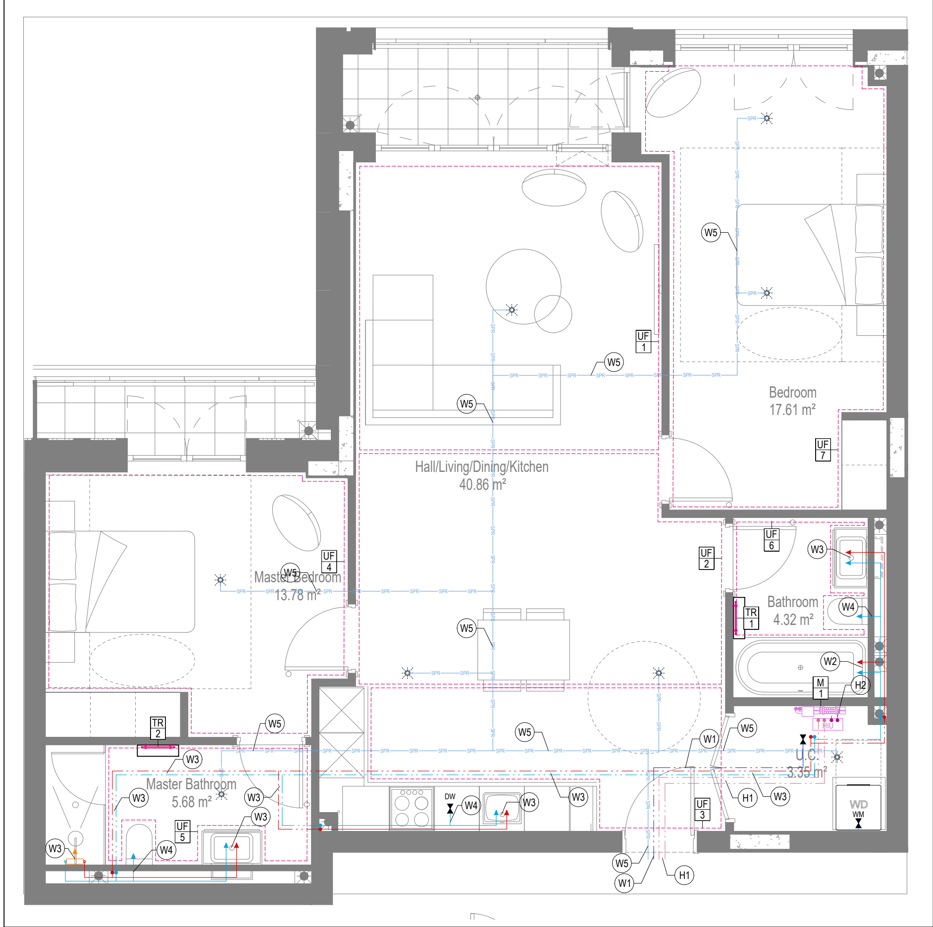
WATER AND HEATING LAYOUT
