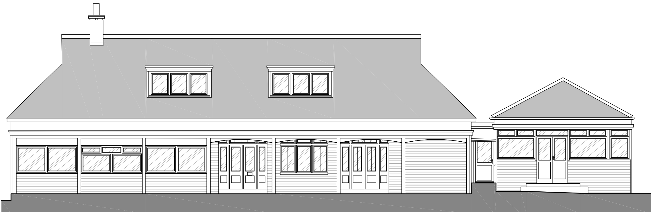
EXISTING FRONT ELEVATION - 1:100
