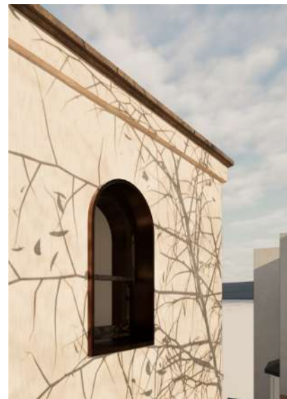
Metal capping + brick band (alternative if weight is an issue)
