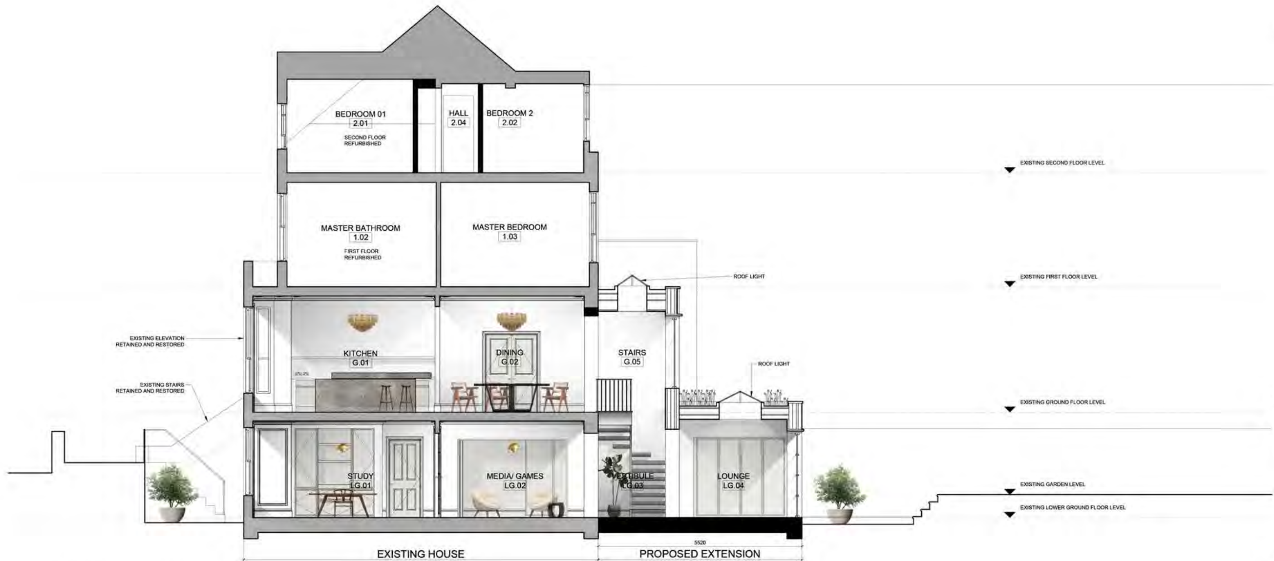
A PROPOSED SECTION Scale: 1:50 SECTION
