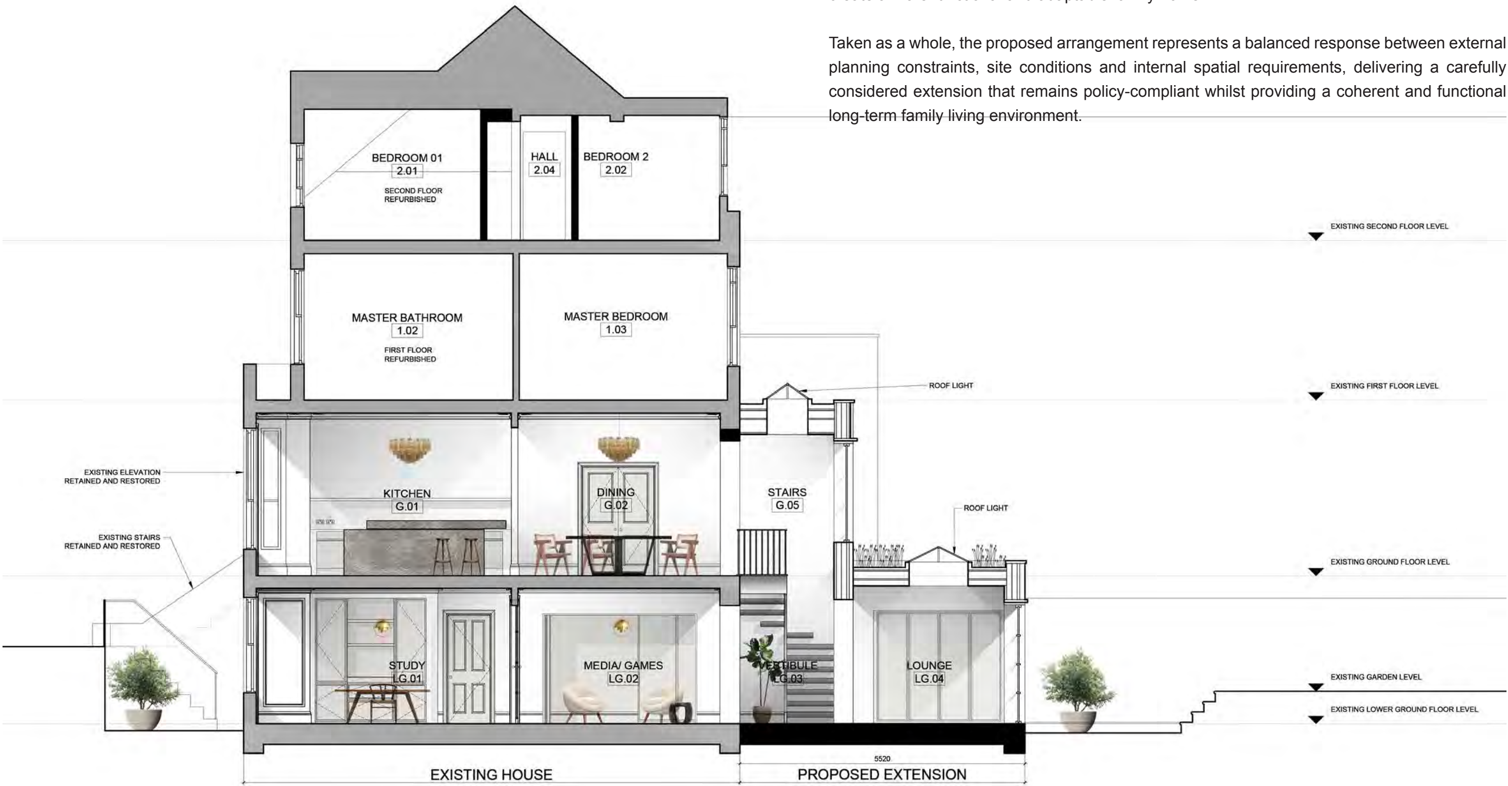
Section of the Proposed Extension in Context of the Existing House
