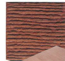
Broached stone tooling (feature))
