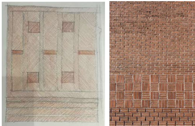
Alternative patterns and materials for ground floor façade masonry. Brickwork (above middle) or Cove Red stone slips (far right).
