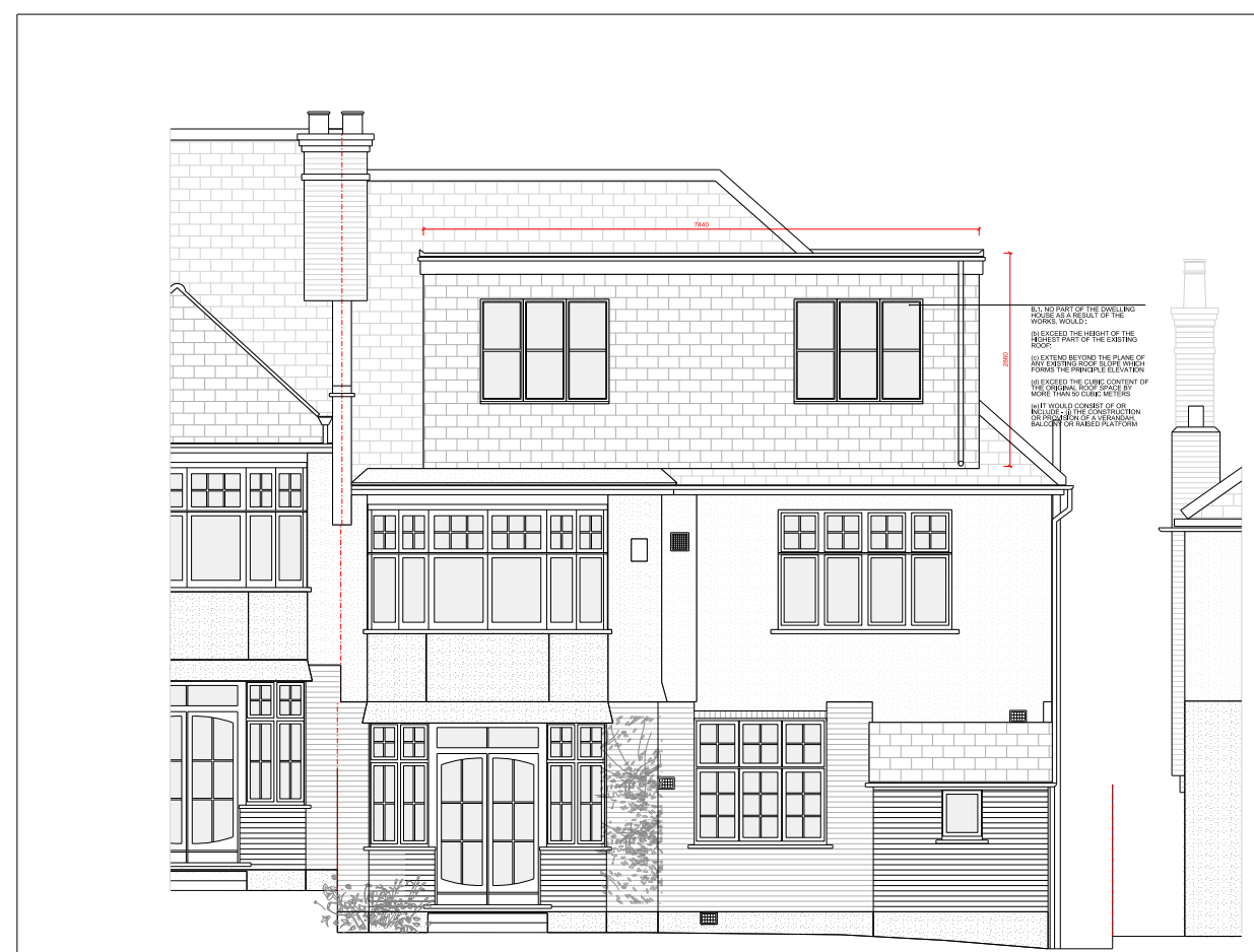
No. 53 Permitted Developmnet - Removed Rear Gable End
