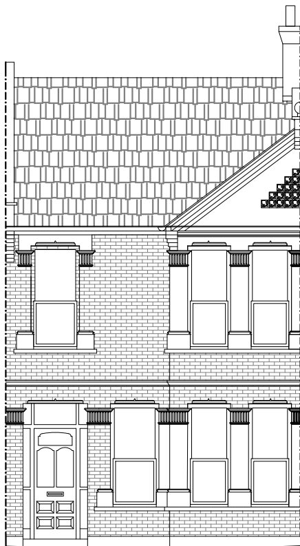
Existing Front Elevation
