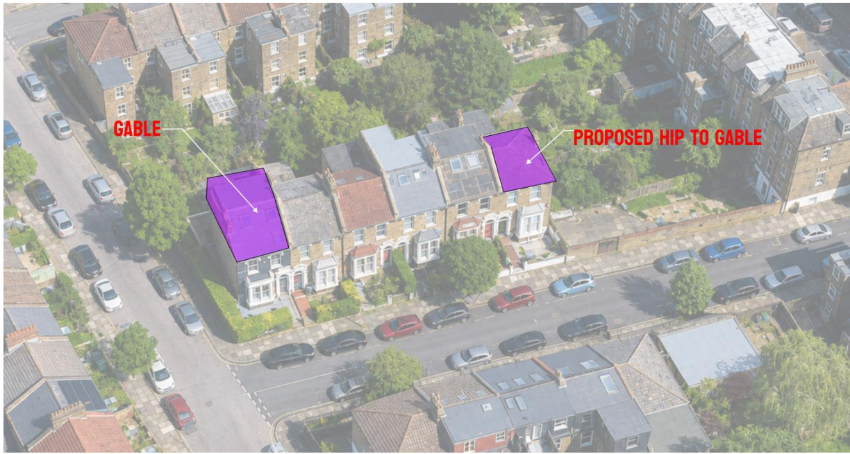
Fig. 5. End of terrace hip to gable roof alteration. Gable roof highlighted in purple (no 12. HGY/2021/1611).
