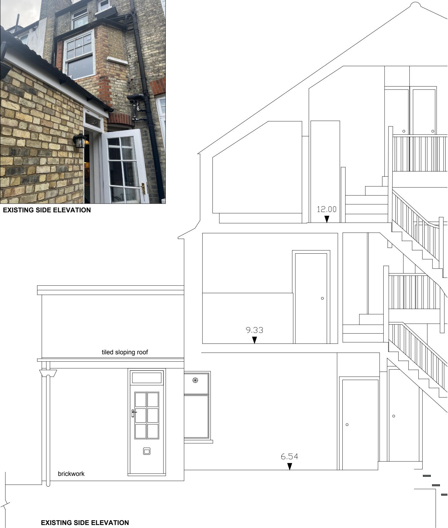
EXISTING SIDE ELEVATION
