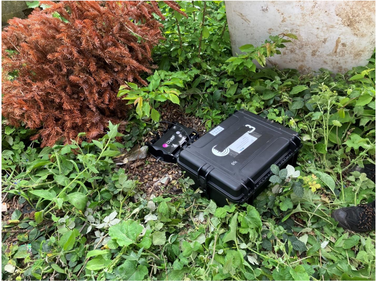
Figure A.4 – Vibration meter at position VP2
