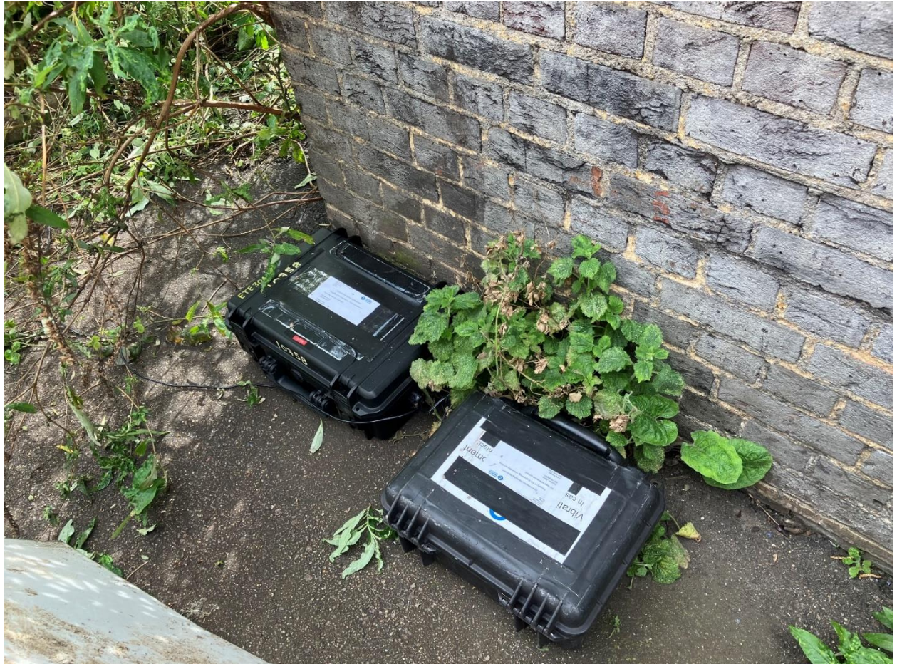
Figure A.3 – Acquisition system and batter for MP5
