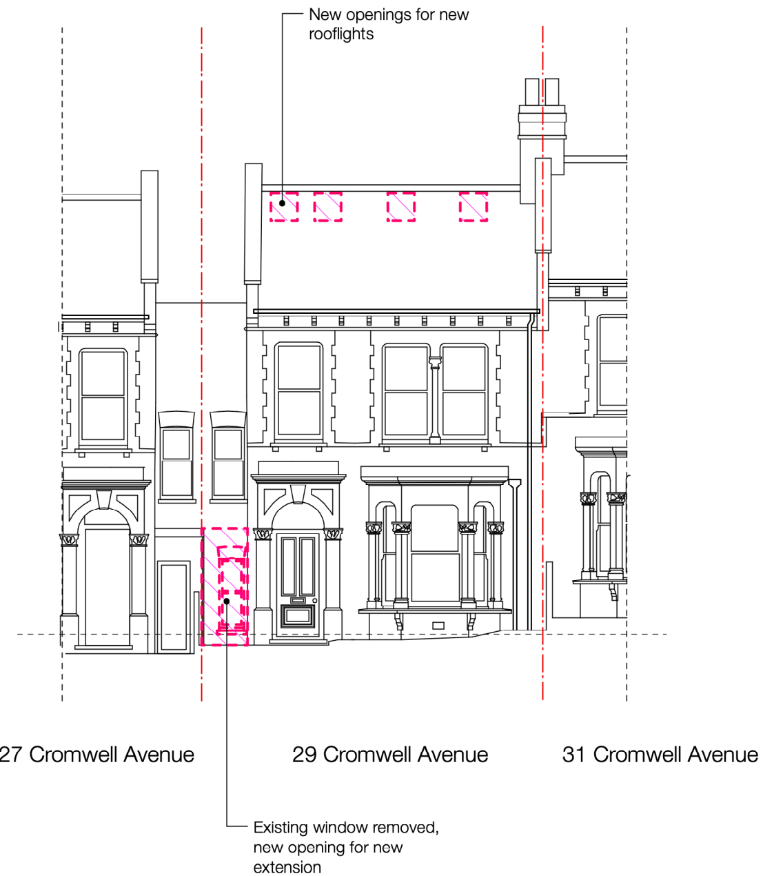
1 Front Elevation - Demolition Scale: 1:100
