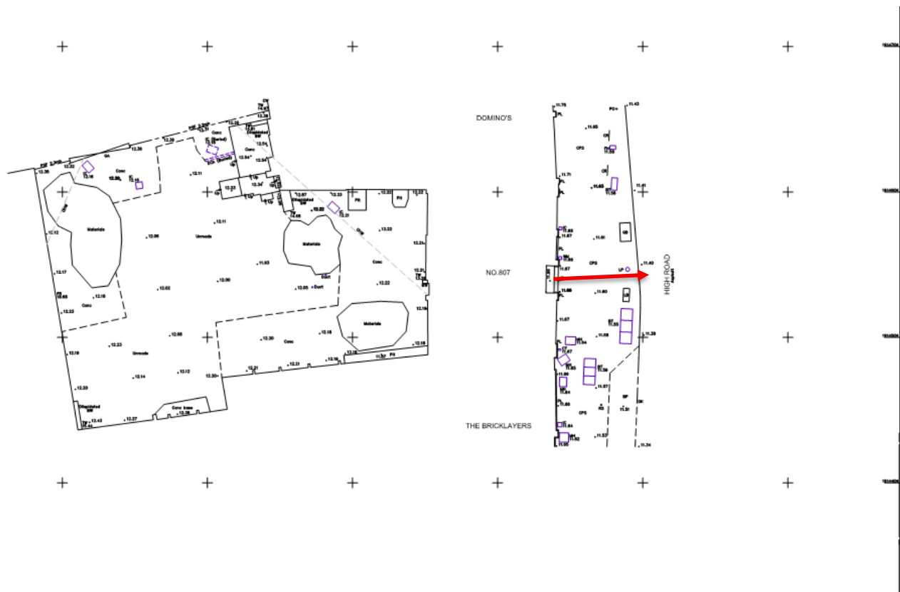
Figure 1 - Topographical Survey indicating overland flow routes
