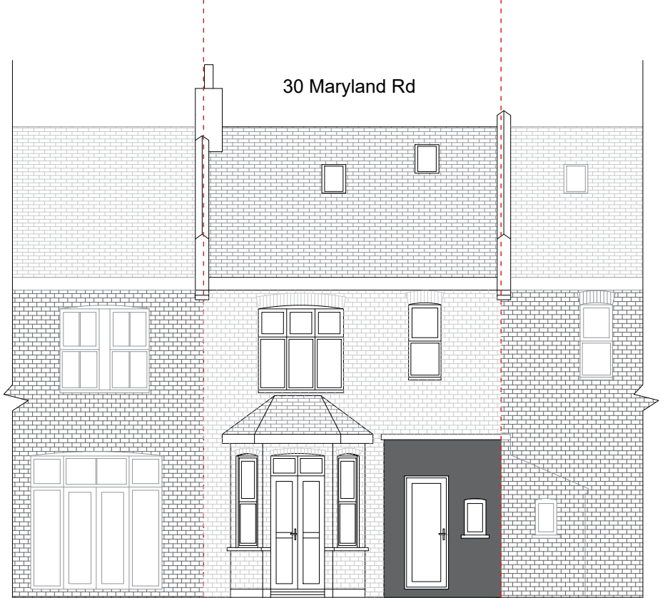
EXISTING REAR ELEVATION
