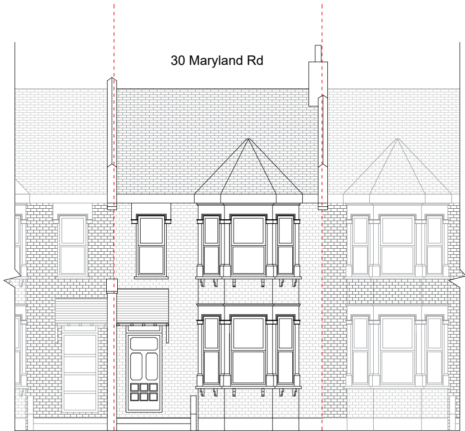
EXISTING FRONT ELEVATION
