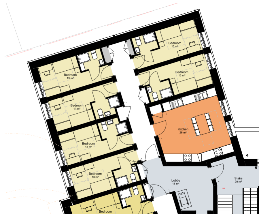
Figure 4 – Kitchen location toward escape end of bedroom corridor
