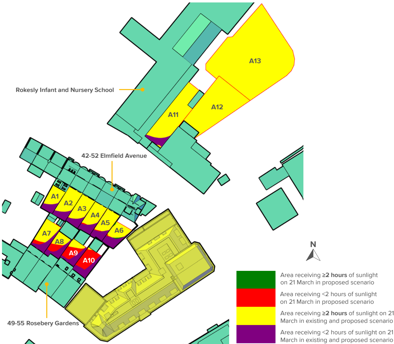
Figure 20: Overshadowing results for existing amenity areas in close proximity to the development site (21 March – BRE criteria)
