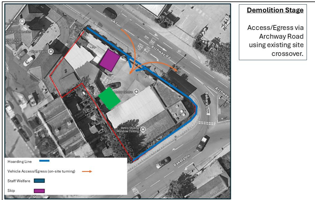
Figure 5.1 Demolition Stage Site Arrangement
