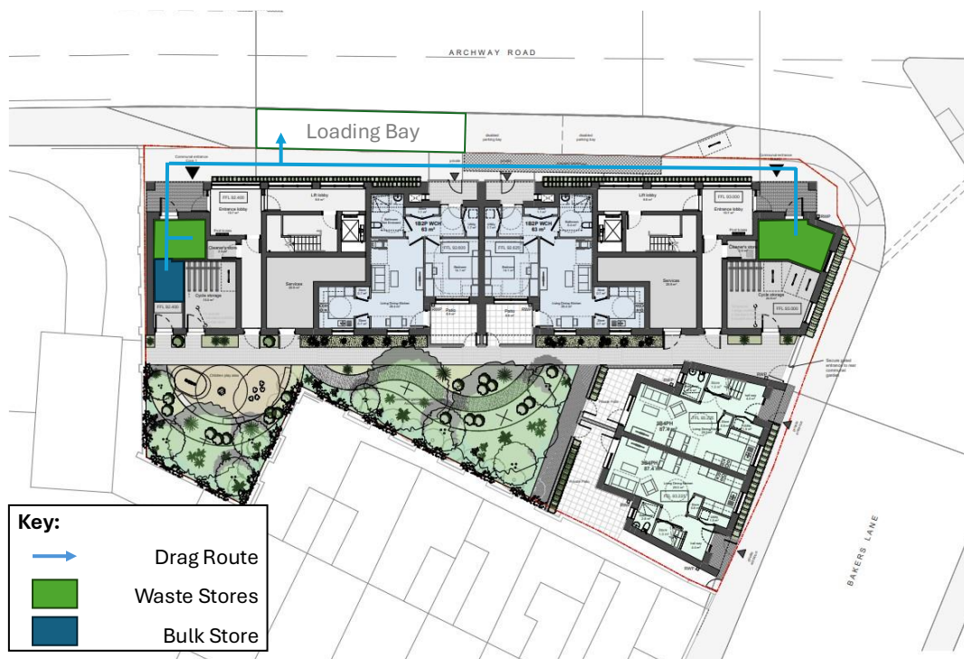
Figure 4.5 Waste Stores Location
