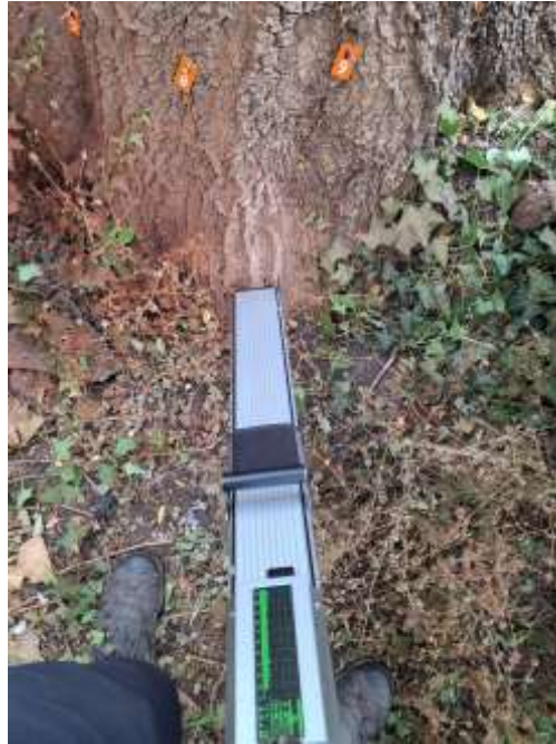
Figure 10: Resistograph drilling in progress in the vicinity of sonic tomography sensor pins 7–9, adjacent to the MP2/MP3 (SE aspect) test locations. (16 August 2026).
