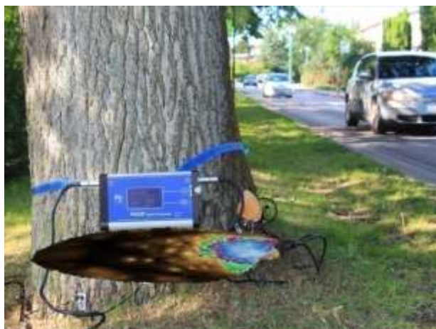
Figure 15: PiCUS 3 Sonic Tomograph in situ on a tree stem. Sensors are connected to small pins inserted into the bark at strategic intervals around the circumference.
