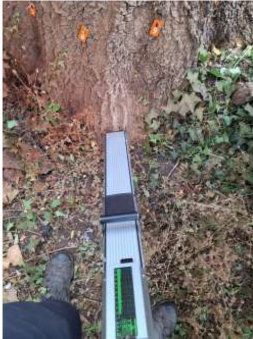
Figure 12: Resistograph drilling in progress in the vicinity of sonic tomography sensor pins 7–9, adjacent to the MP2/MP3 (SE aspect) test locations (same photograph as MP2, above). (16 August 2026).
