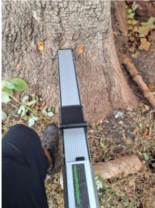
Figure 16: Resistograph drilling in progress in the vicinity of sonic tomography sensor pins 14–15, adjacent to the MP5 (NW aspect) test location. (16 August 2026).
