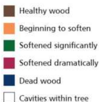
Figure 16: PiCUS Sonic Tomography colour legend. Colours represent relative sound velocity as a proxy for wood condition: brown = healthy wood; orange = beginning to soften; dark green = softened significantly; pink = softened dramatically; dark blue = dead wood; white/light blue = cavities.
