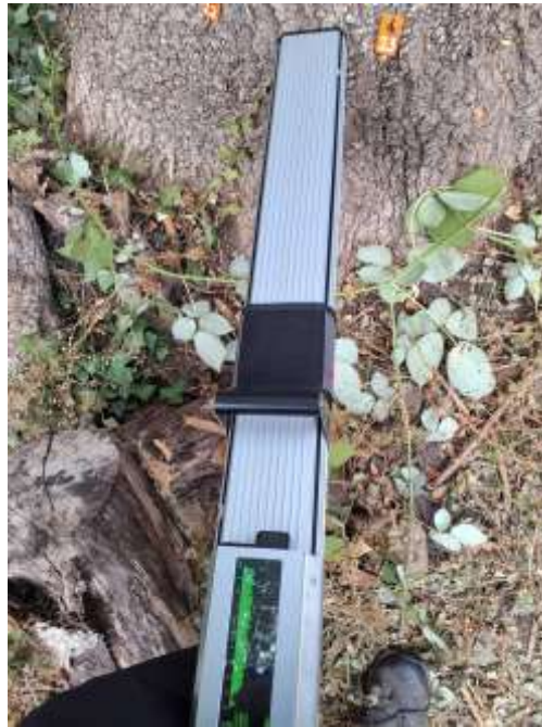
Figure 14: Resistograph drilling in progress in the vicinity of sonic tomography sensor pins 12–13, adjacent to the MP4 (NE aspect) test location. (16 August 2026).
