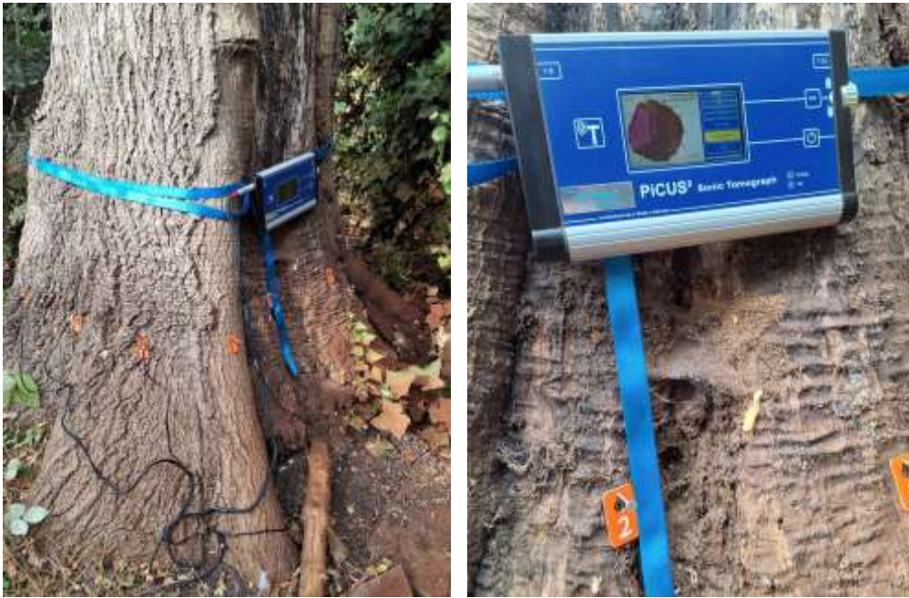
Figure 6: PiCUS 3 sensor array installed on T001 prior to sonic tomography (left), and the PiCUS 3 display showing the tomogram being captured in real time on site (right), 16 August 2026. Numbered sensor pins correspond to the positions shown in Figure 5.
