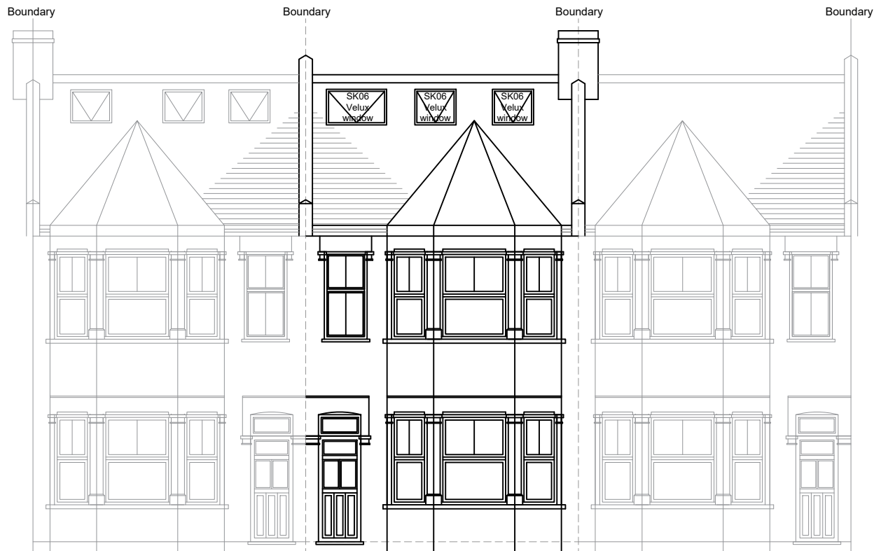
PROPOSED FRONT ELEVATION SCALE 1:100
