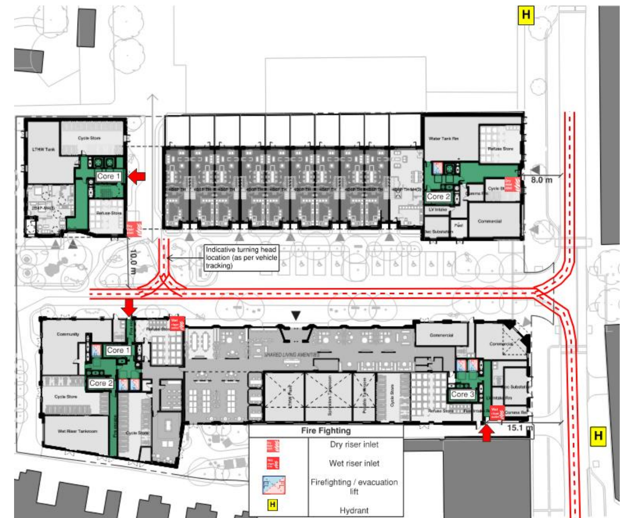
Figure 20 - FRS access and firefighting provisions
