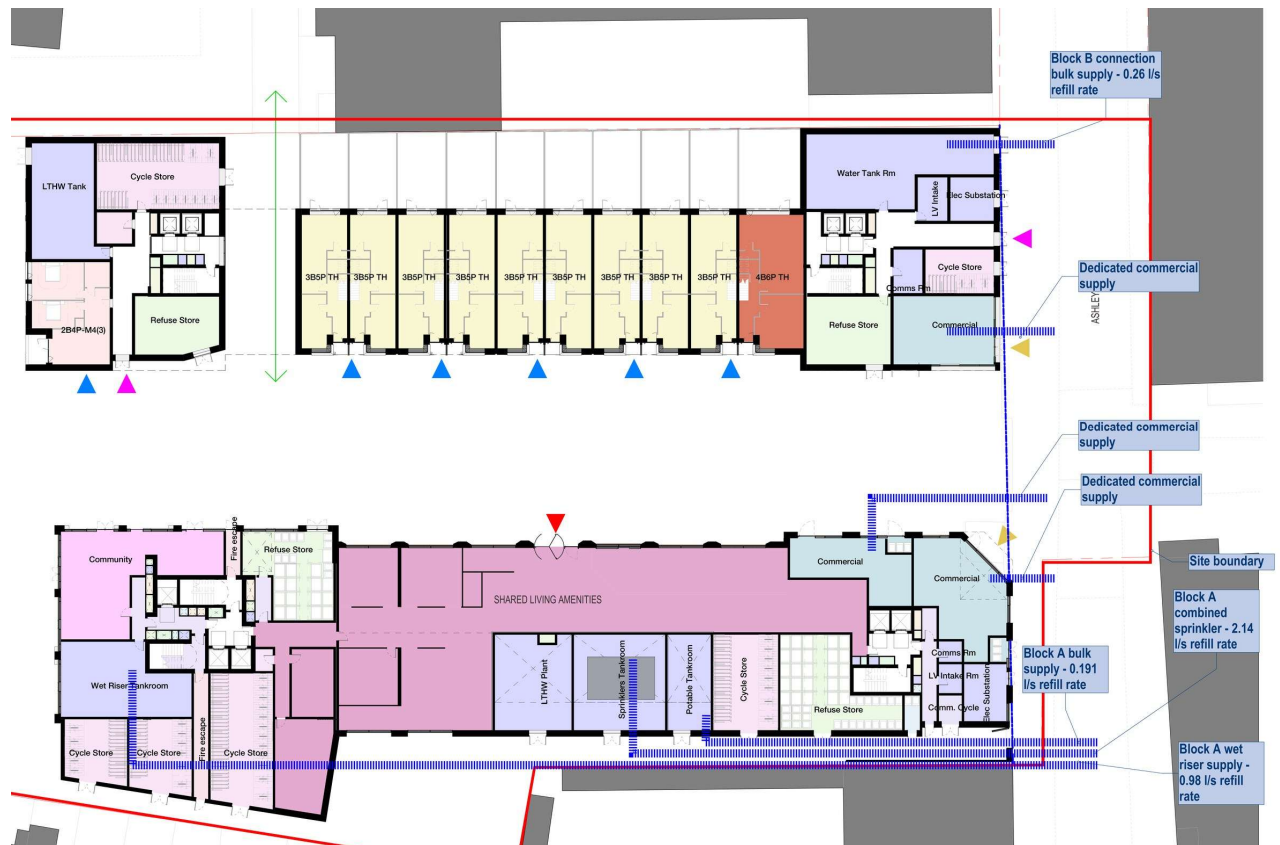
Figure 8-1: Proposed water connection points and refill rates
