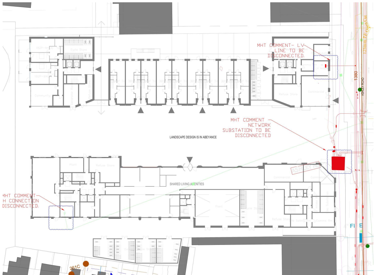
Figure 6-1: Existing utility overlay, showing the assets to be disconnected
