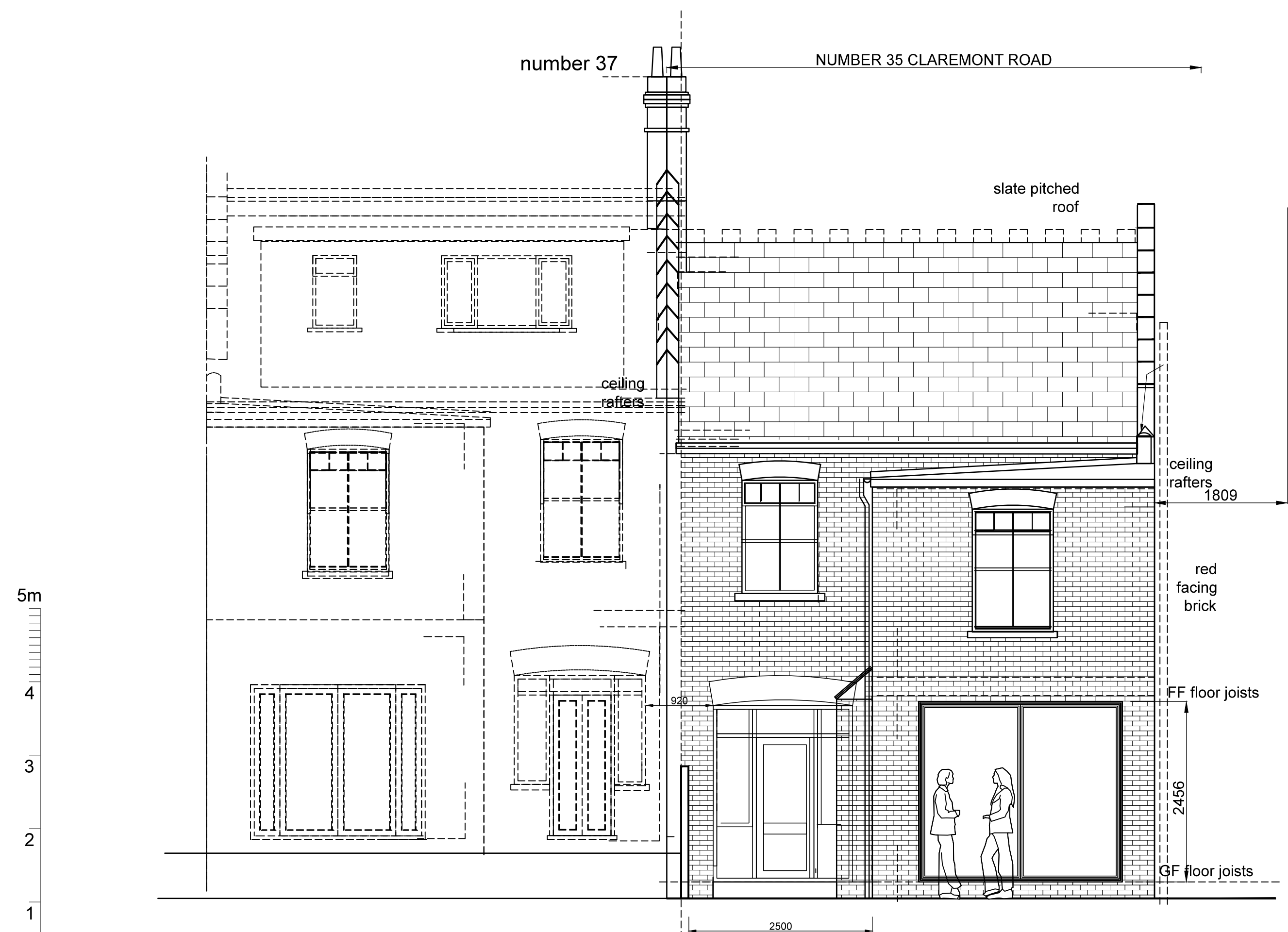
rear elevation as existing scale 1-100@ A3. 1-50 @ A1
