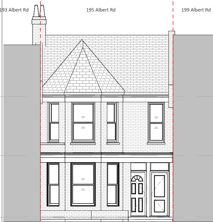
Existing Front Elevation
