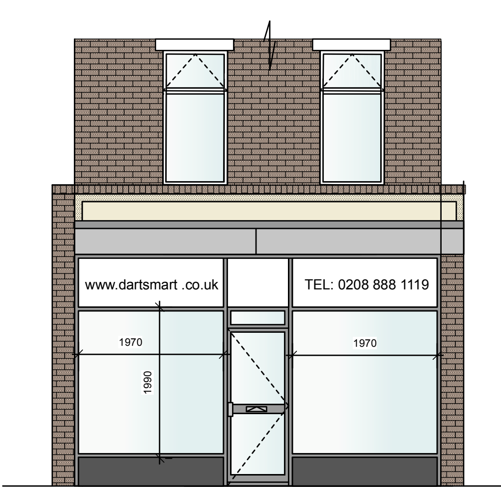
Existing main road elevation
