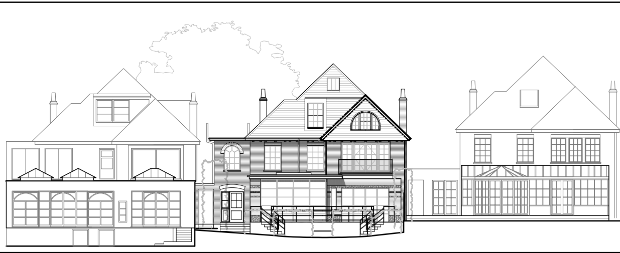
Elevation showing extents of neighbouring rear extensions
