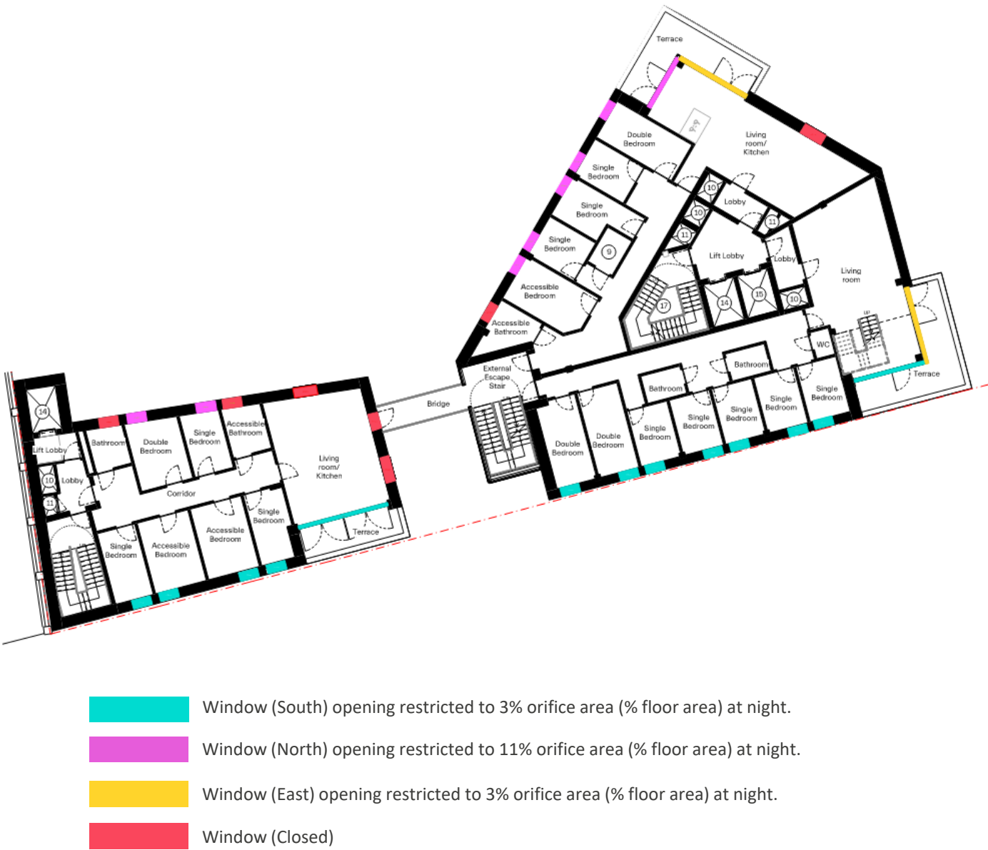
Figure 3: Mark-up indicating locations with restricted window openings due to external noise
