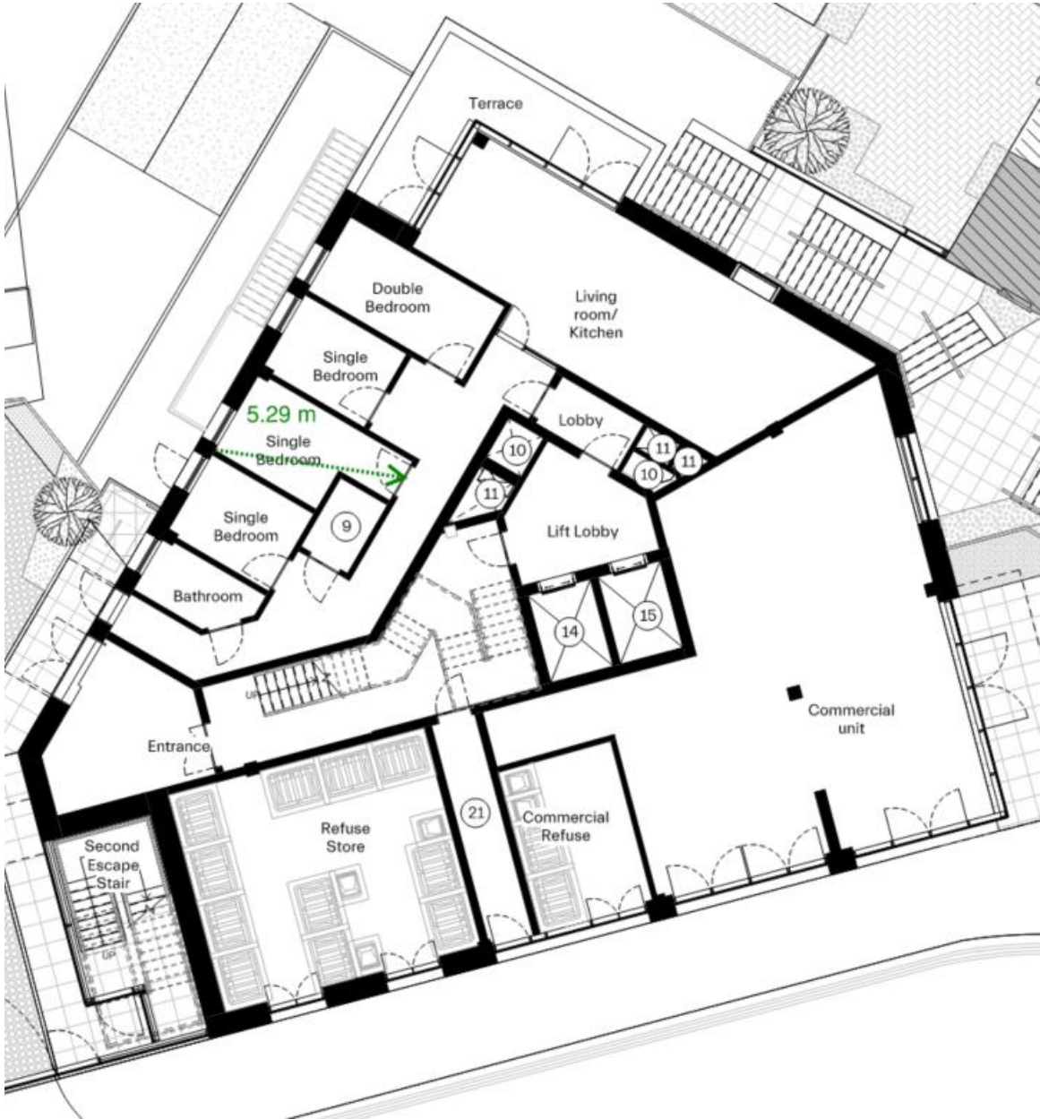
Figure 9.1 Maximum dwelling direct distance on the ground floor (Block A)
