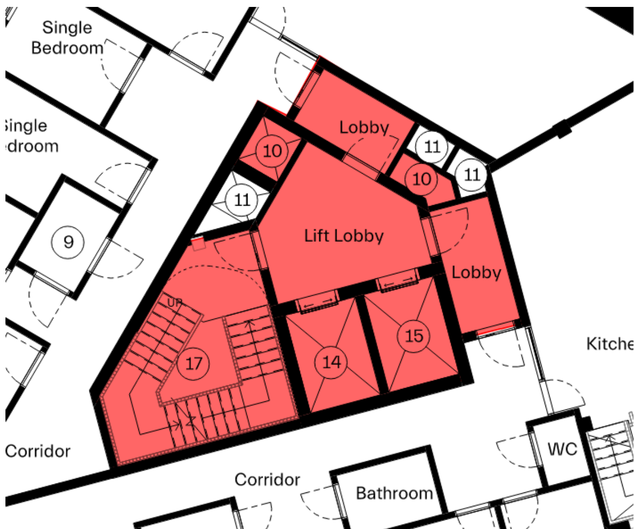
Figure 8.3 The firefighting shaft, highlighted in red.
