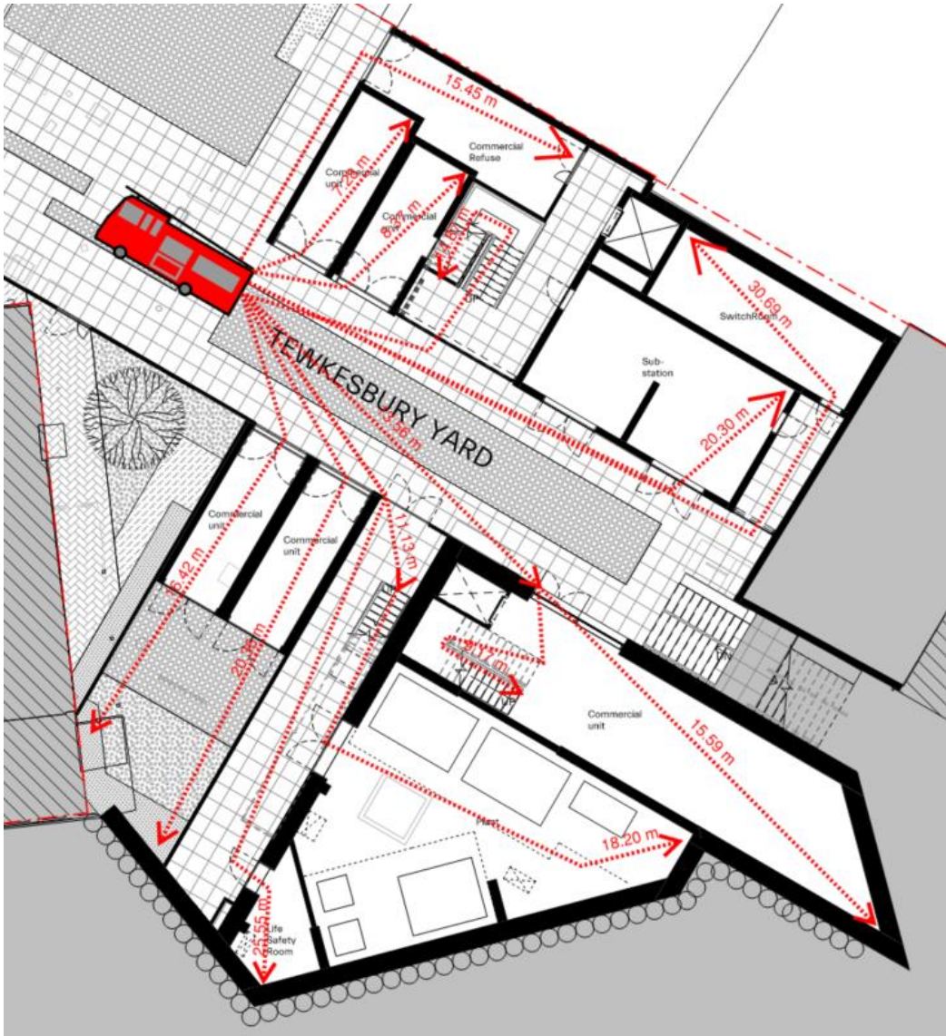
Figure 9.13 Hose distances for the Tewkesbury Level
