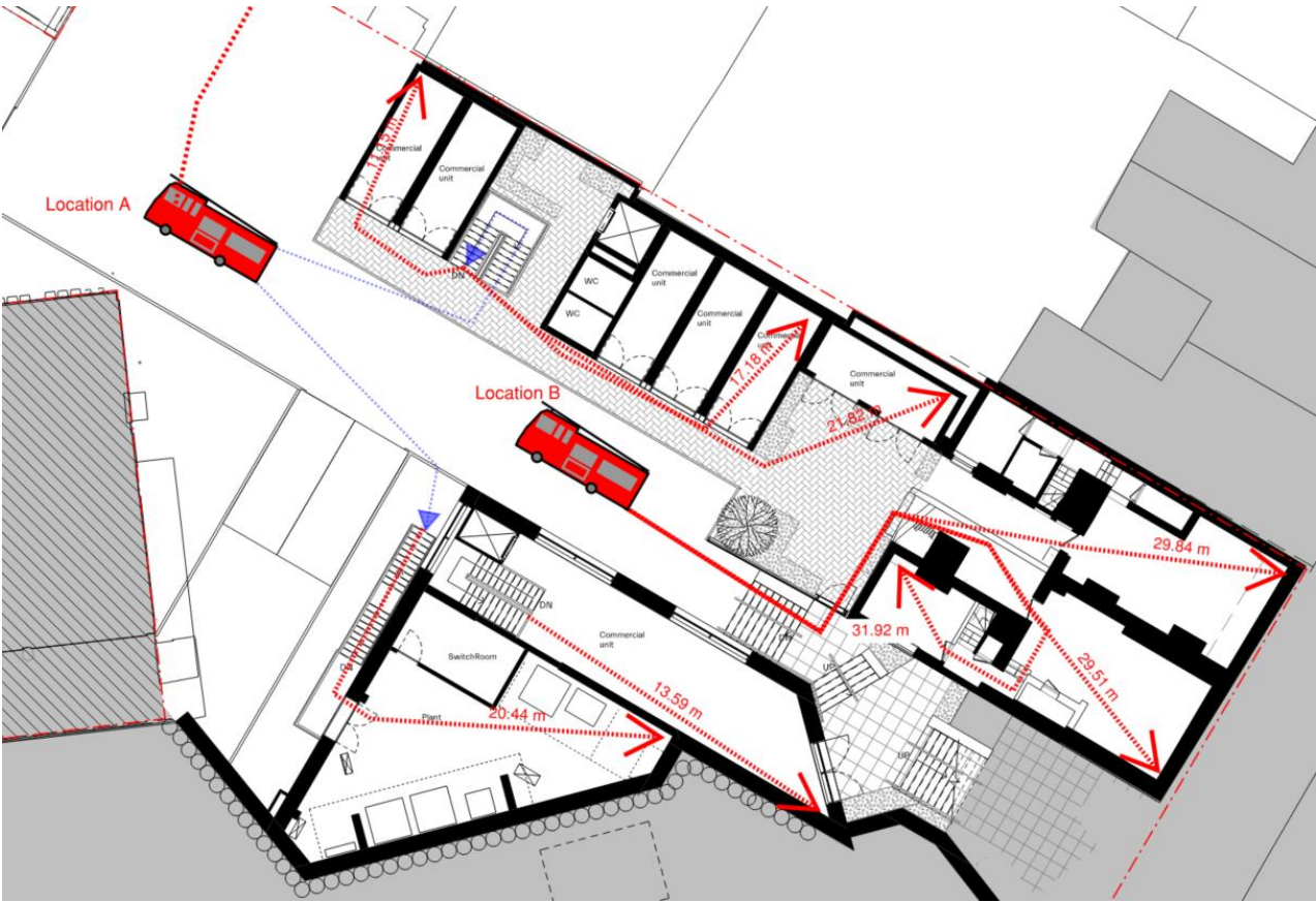
Figure 9.14 Hose distances for the mezzanine at Tewkesbury Level
