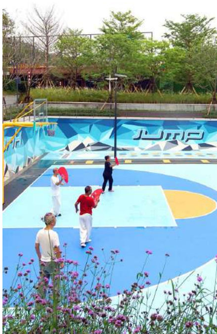
Basketball and netball courts - Porous asphalt with coloured anti slip coating
