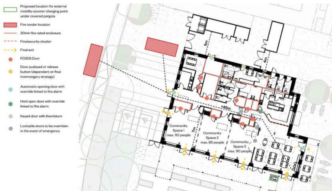
Figure 14: Proposed Fire Strategy - Extract from 21.07.2023 Fire strategy Note Levitt Bernstein & Toga Fire
