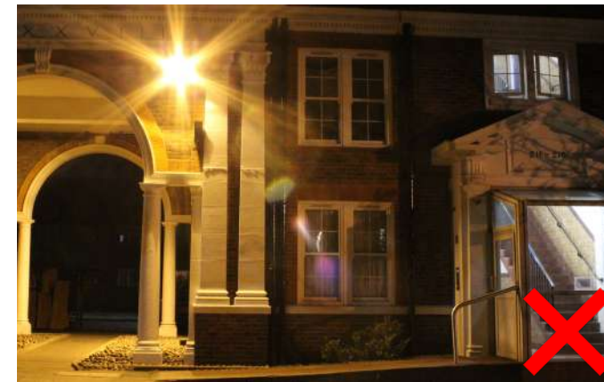
Uncontrolled light optics such as bulkheads to be avoided
