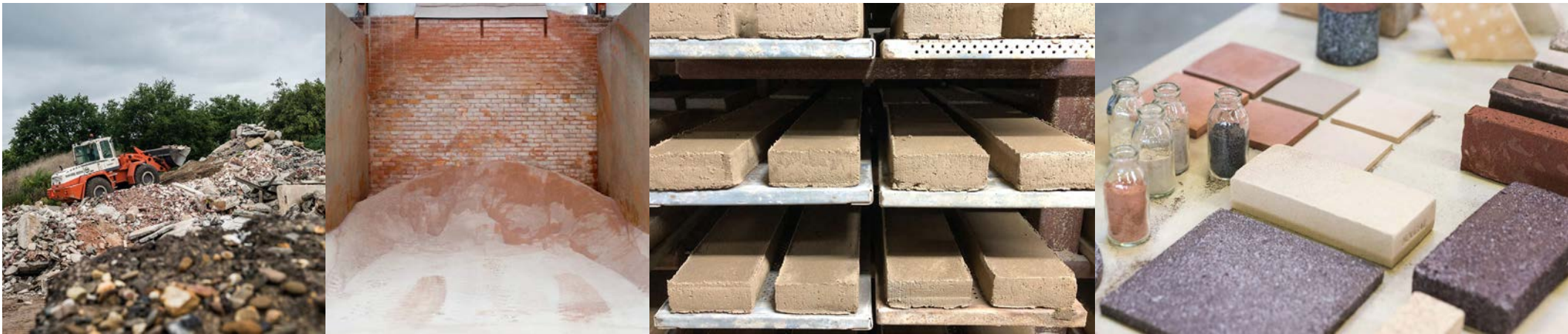
Process of making waste based bricks at Stonecycling
