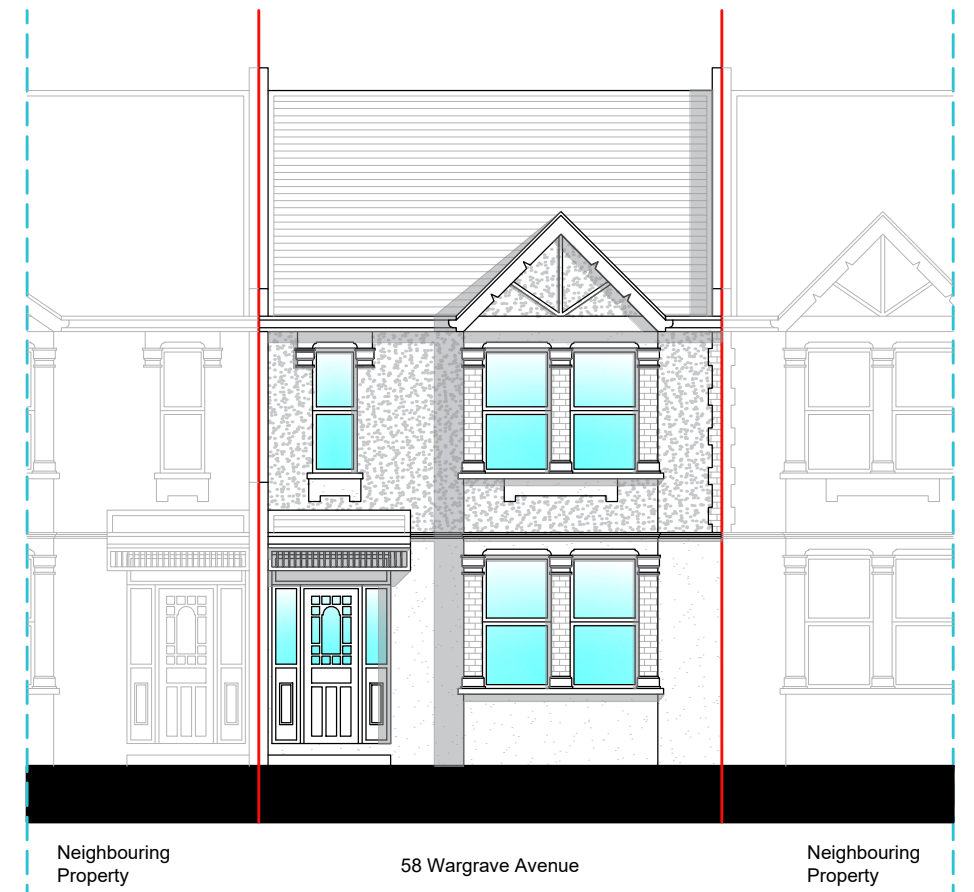
EXISTING NORTH-WEST ELEVATION (FRONT VIEW)
