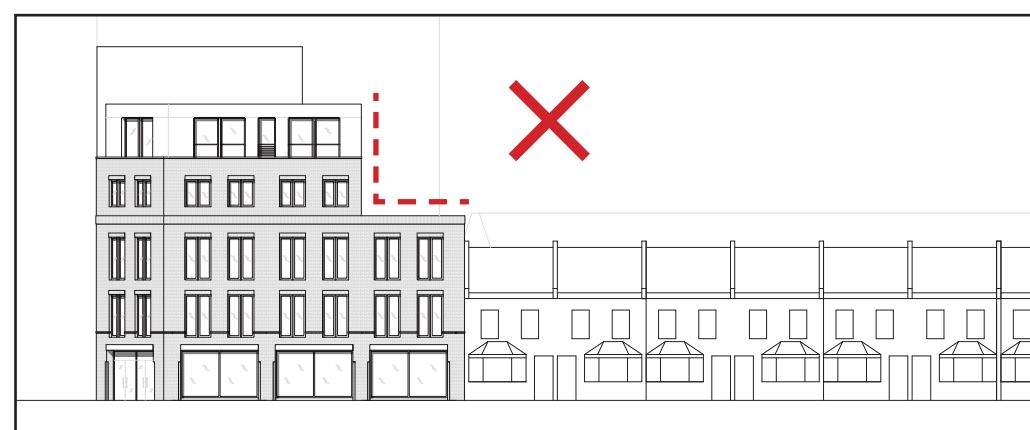
FIGURE 05 - EXTENDED STEP AWAY FROM ESIN COURT AT THIRD FLOOR APPEARS AWKWARD
