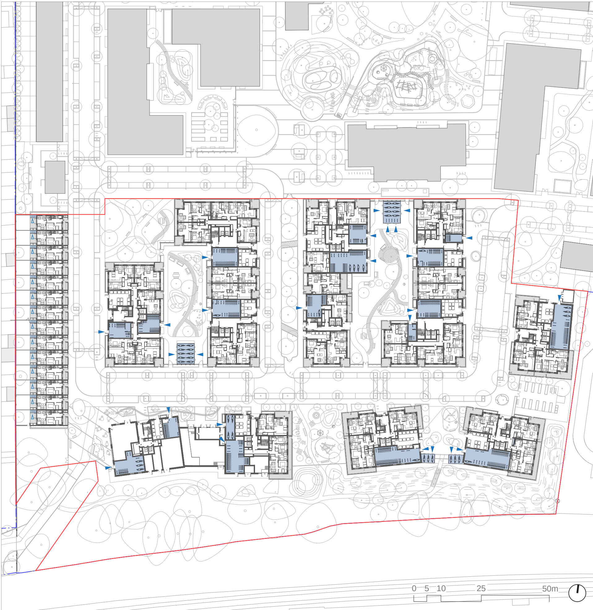
Ground floor showing cycle store locations
